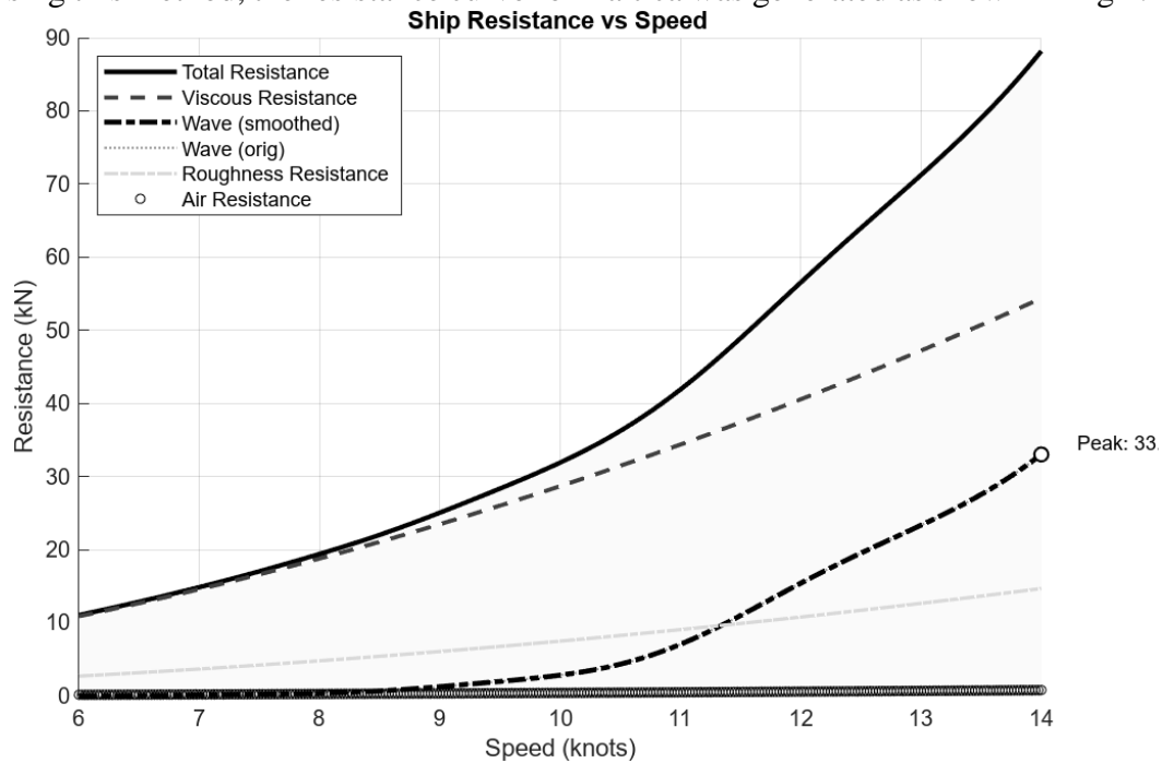
Fig 2.12: Resistance curve for M V Baltica
