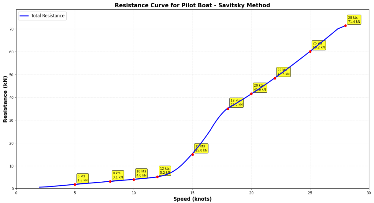
Fig 2.10: Resistance curve for the pilot boat hull by Savitsky method
