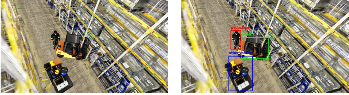
Figure 4.11: Comparison of the original image (left) and the same image with 2D bounding-box annotations over the detected actors (right).
