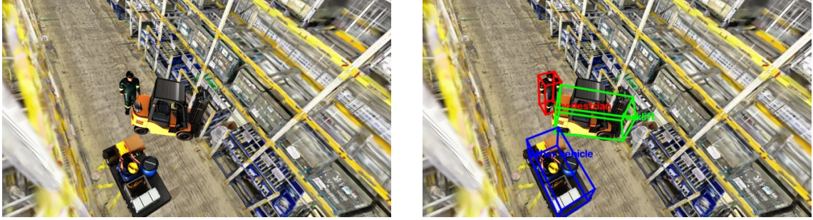
Figure 4.10: Comparison of the original image (left) and the same image with 3D bounding-box annotations surrounding the detected actors (right).
