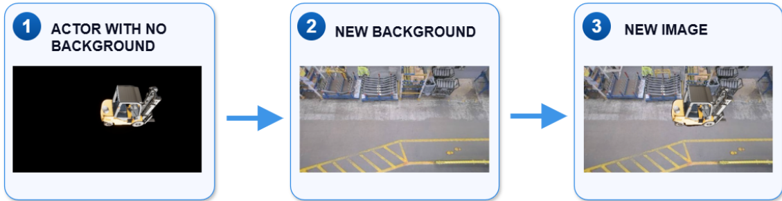
Figure 3.3: Cut-and-Paste procedure for simulated objects.
