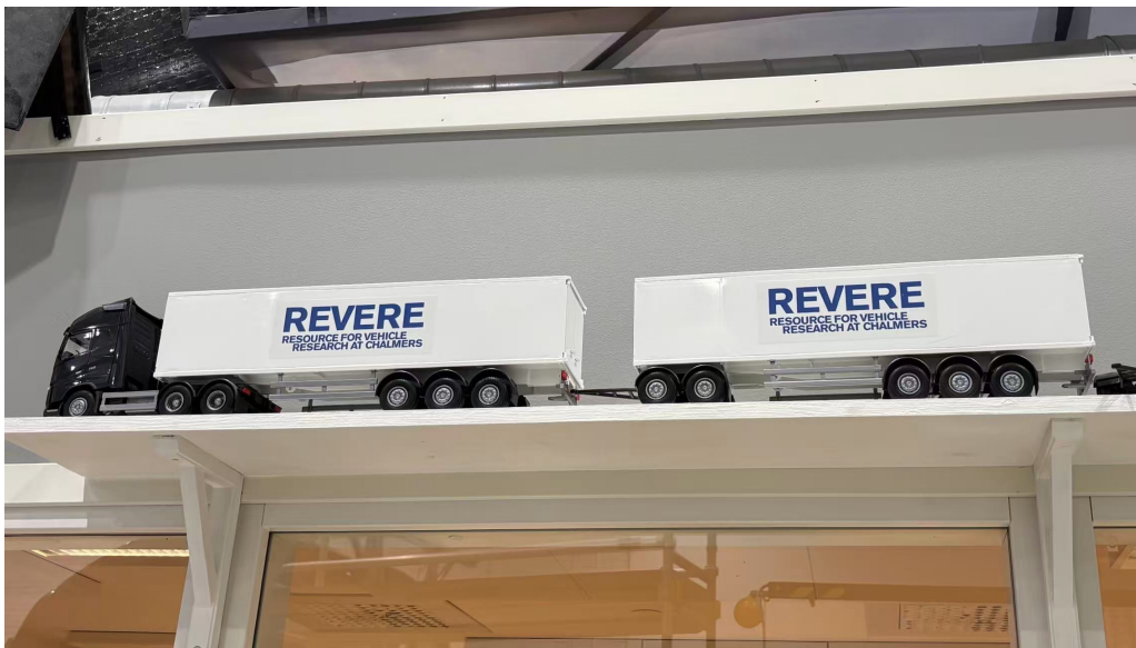
Figure 1: A-double scaled model (REVERE)
