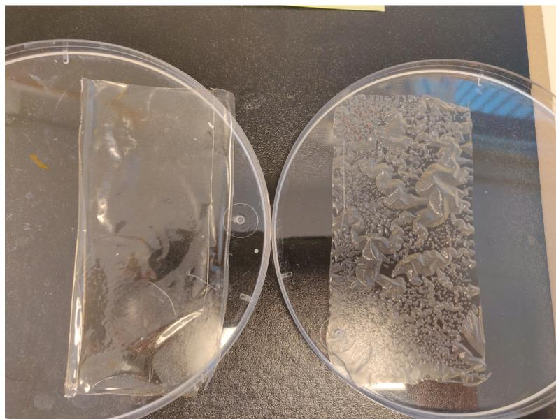
**Figure 4.5:** Comparison between OX/PVA/sorbitol films stored for 72h at (left) 30% and (right) 90% RH.
