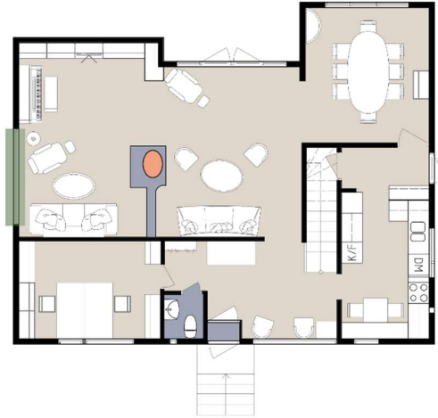
Figure 1 Materials and details that might be commented on during an interview. Original floors marked in brown, marble floors and countertop in blue/grey, a stained-glass window in green, and the oval chimneypiece in orange.
