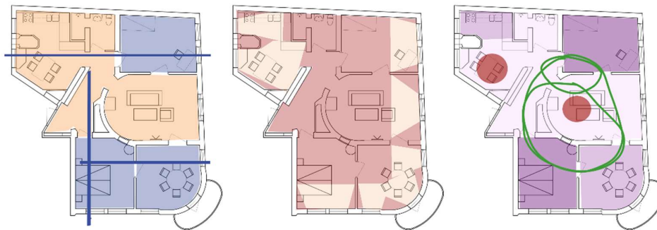
Figure 16 This apartment has more flexibility in the rooms, but the plan is still closed. The central hallway is very dark, but provides several access points and connections between the rooms. All the doors make the division of public and private easy.
