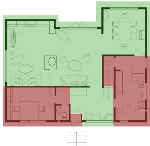
Figure 2 A diagram showing the difference in closed vs open areas of a plan, open areas have large or no doorways, closed areas are narrow or secluded.
