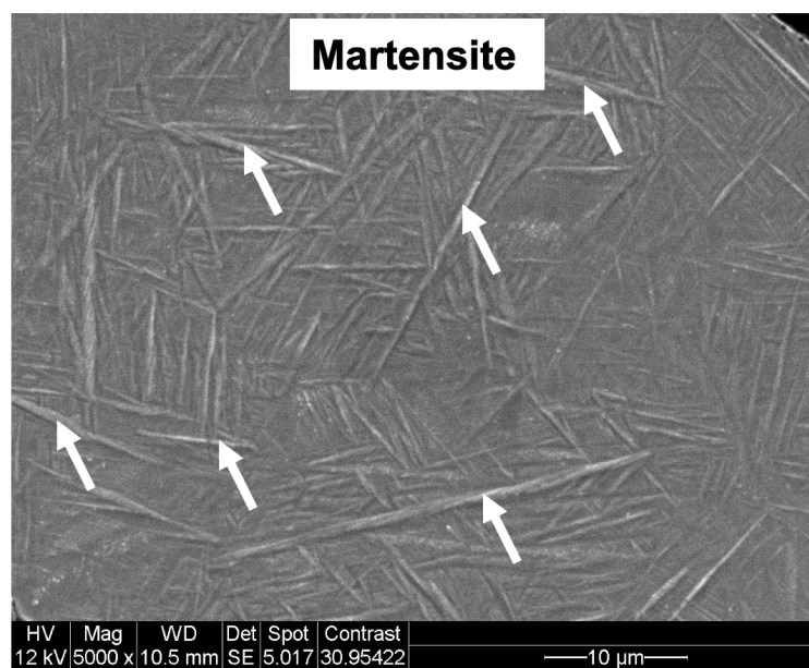
Figure 53: ESEM image of the virgin powder's microstructure.
