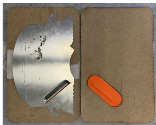
Figure 8.8: Setup for pressing the louvre into filter holder using 3D-printed tool and laser-cut MDF.
