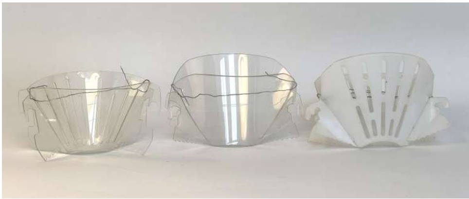
Figure 8.9: Three generations of laser-cut plastic filter holder prototypes. Held in tension using a metal wire.
