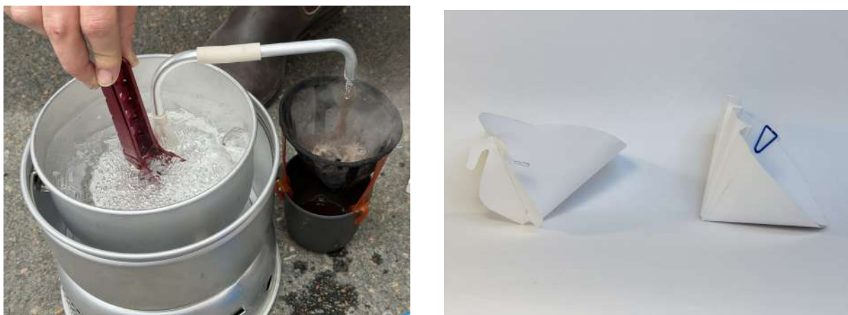
Figure 7.6: Left: First Auto Drip prototype tested with the GSI Pour Over as filter holder. Right: Early Auto Drip filter-holder prototypes made out of paper.
