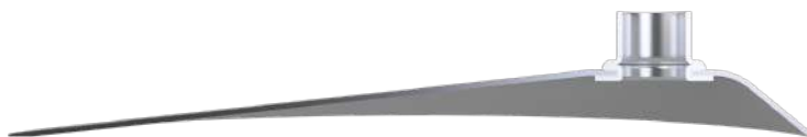
Figure 9.7: The pump base in a cross-section view showing how the small protrusion is riveted.
