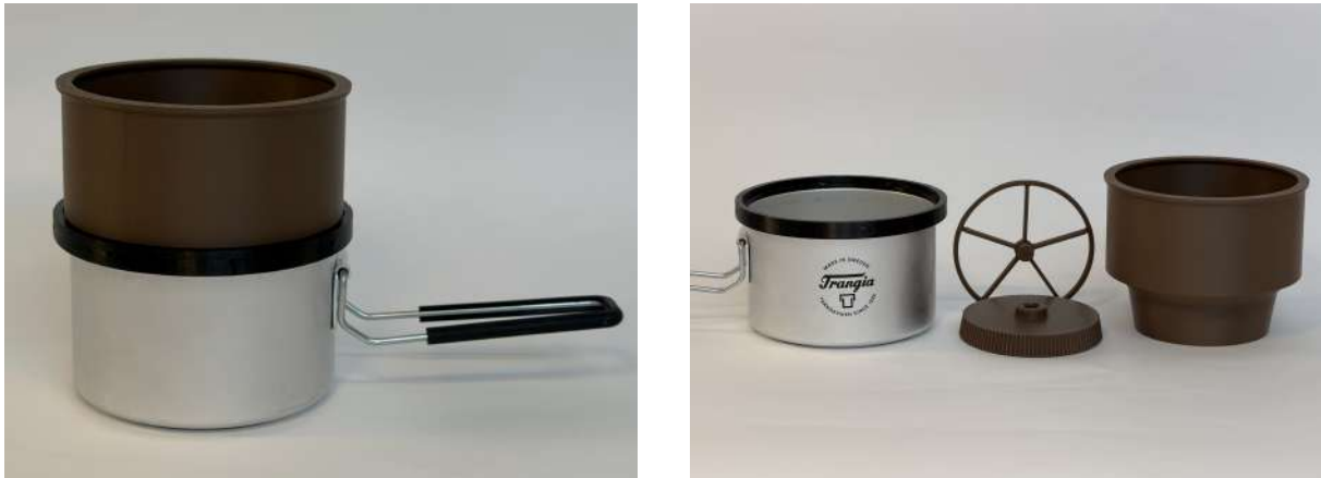
Figure 7.8: Vacuum Top test rig assembled (left) and disassembled (right).
