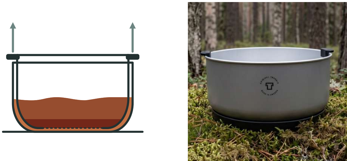
Figure 7.18: Left: Illustration of the brewing principle, showing how the coffee is separated from the coffee grounds. Right: Concept rendered in a potential use environment, created using generative AI (Google, 2026).
