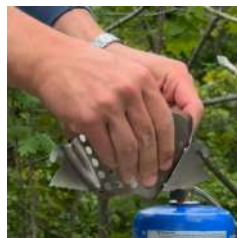
6. Slot other side of filter holder.
