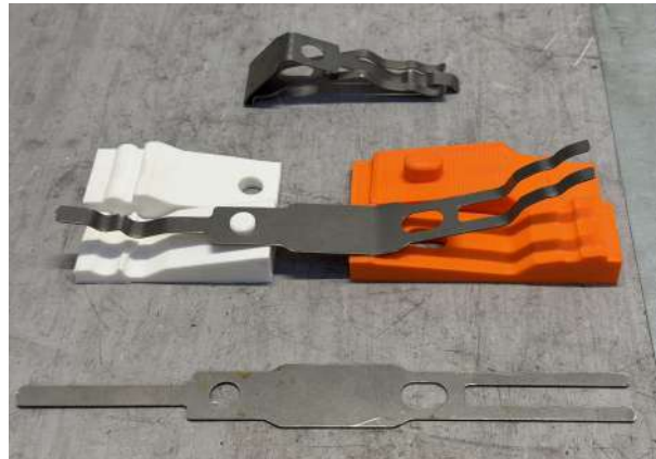
Figure 8.7: Bending sequence of clip prototype using 3D-printed tools.
