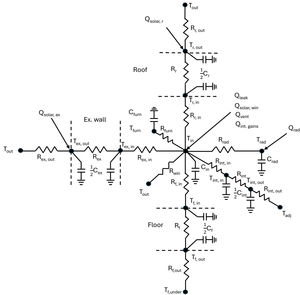
Figure 4.5: Circuit for one zone in a building
