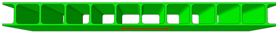
Figure 5.16: Path on the bottom surface under unloaded (left) and loaded (right) cell.
