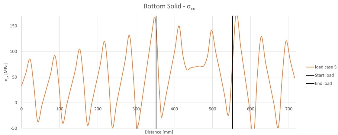
Figure 5.20: Normal stress distribution in x -direction for the bottom surface of the solid model, load case 5. Distance [mm] on the x -axis and stresses [MPa] on the y -axis.
