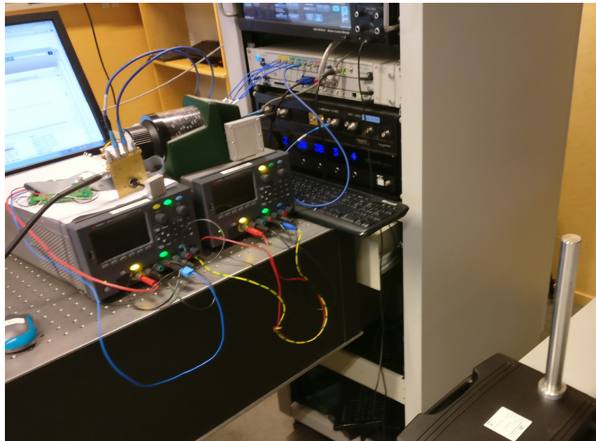
Figure 4.11: Lab setup used by both the MSK-LFM and OFDM radar for measuring different kind of target setups. In this case a single metal pillar is placed roughly 1 m from the transceiver.
