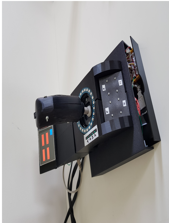
Figure 3.32: The drawer underneath the test bench with the purpose of hiding away components and enabling hot switching.
