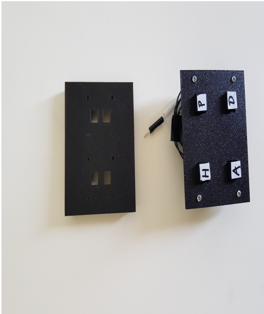
Figure 3.22: The plates that were to house the different activation components were made to be the same size as the touchscreen.
