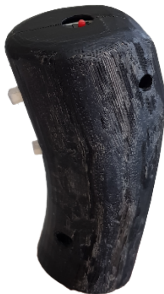
Figure 4.7: Tactile push buttons, placed in the joystick handle.
