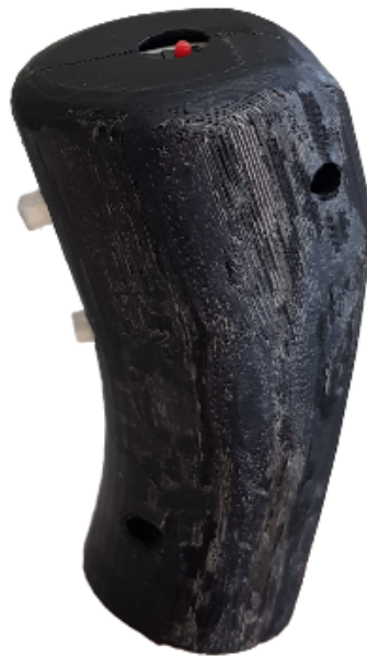
Figure 4.15: The strongest concept in Scenario 3 - Tactile push buttons, placed in the joystick handle.
