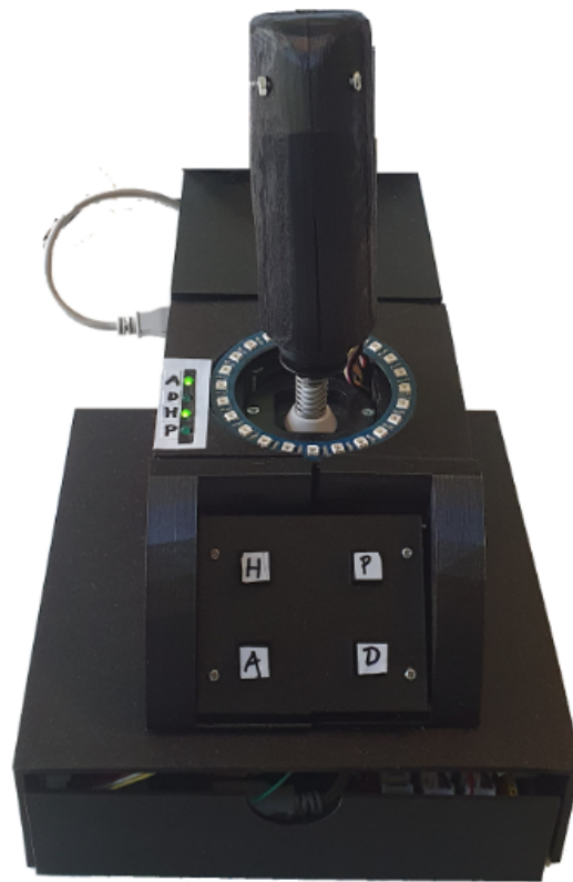
Figure 4.11: The strongest concept in Scenario 1 - The joystick with tactile buttons, placed on the joystick base.
