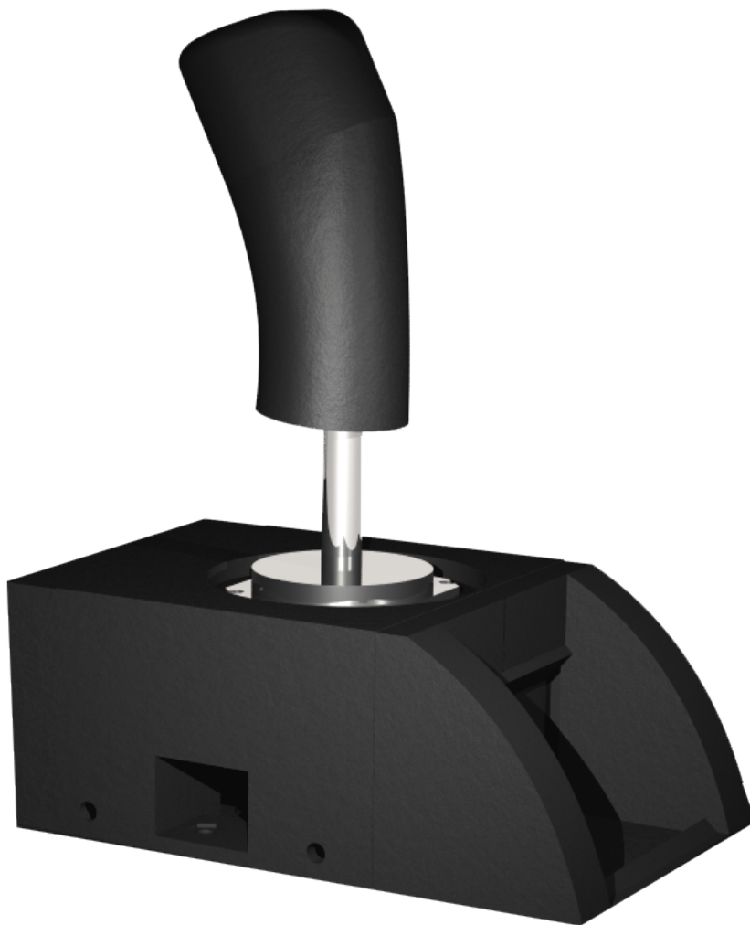
Figure 3.19: The test bench with the metallux joystick, centerpiece, handle and a module.
