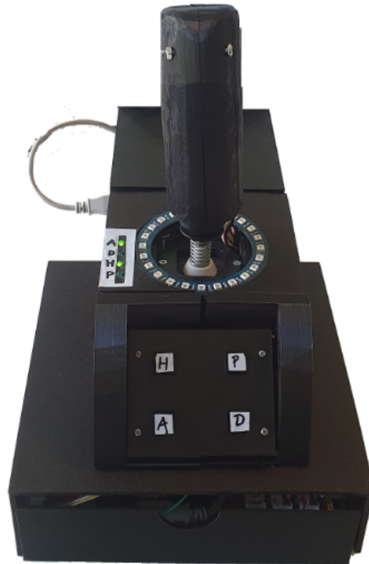
Figure 4.4: The joystick with tactile buttons, placed on the joystick base.
