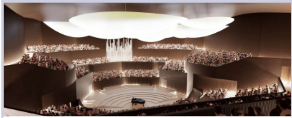
With a volume of around 25 000m³, the concert hall can accommodate 2348 seated visitors, excluding the positions reserved for wheelchair. The seats are predominantly placed in front of the stage less than 30m away, creating a closer interaction for all listeners. A fundamental advantage of the vineyard style, besides offering a theatrical experience.
