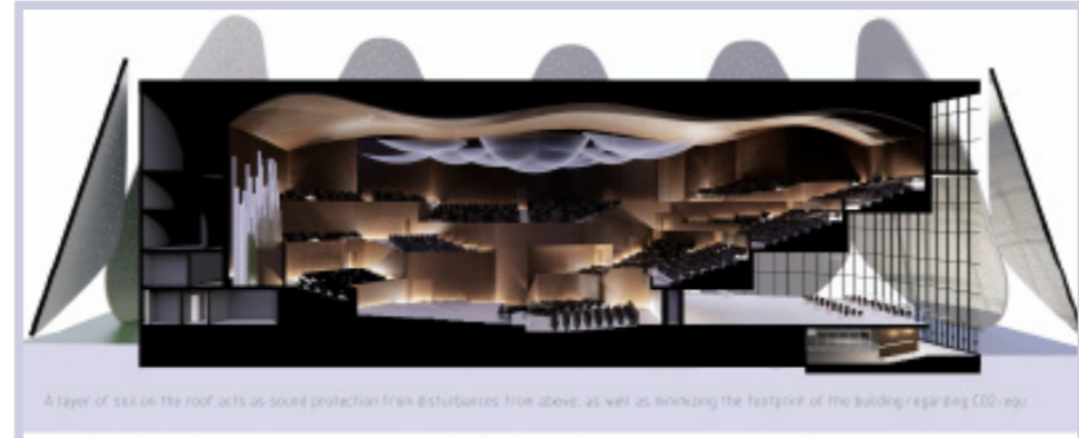
A layer of soil on the roof acts as sound protection from disturbances from above, as well as winning the footprint of the building regarding CO2-equ.
