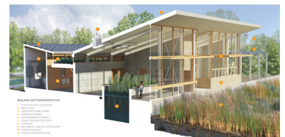
Figure 7.13. Water treatment system in Omega
