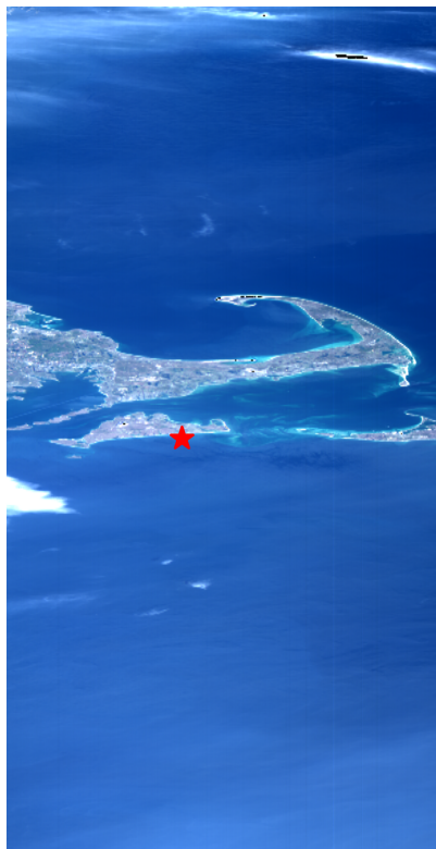
Figure D.1: RGB plot of (uncorrected) ToA reflectance from HYPSONO-2 capture over "MVCO" validation site in Massachusetts, USA, with AERONET-OC validation site marked with a red star, and saturation mask in black, on 2025-04-10.
