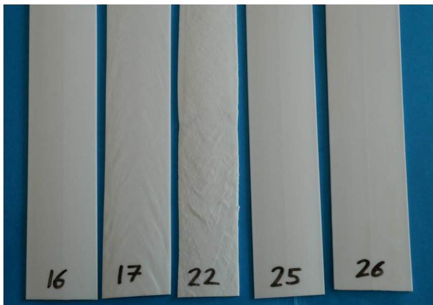
Figure 4.6: Tapes made with polymer B and different CMBs, marked with tape numbers.
