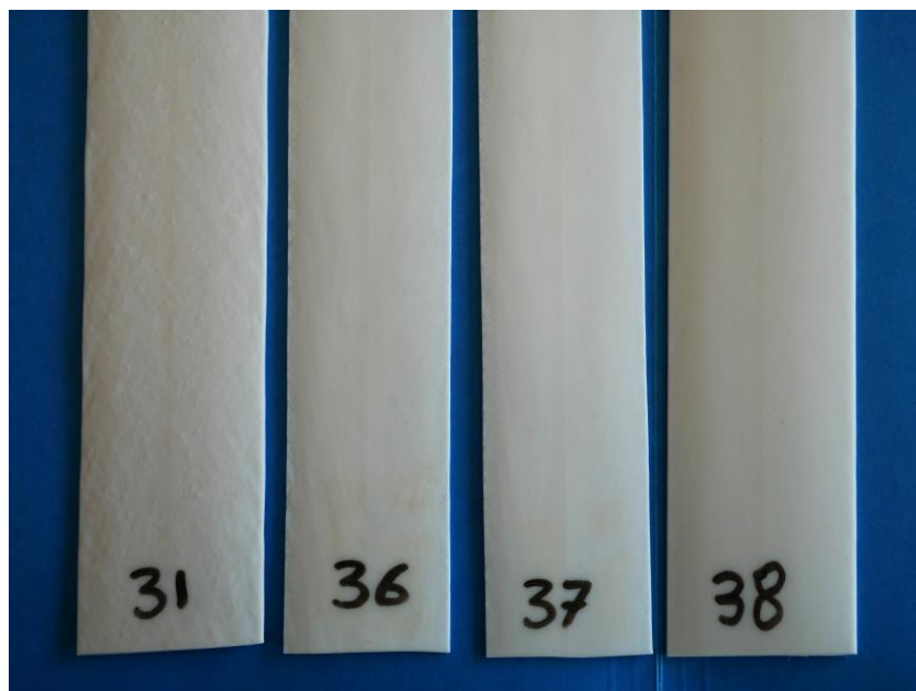
Figure 4.9: Tapes made with polymer C and different CMBs, marked with tape numbers.
