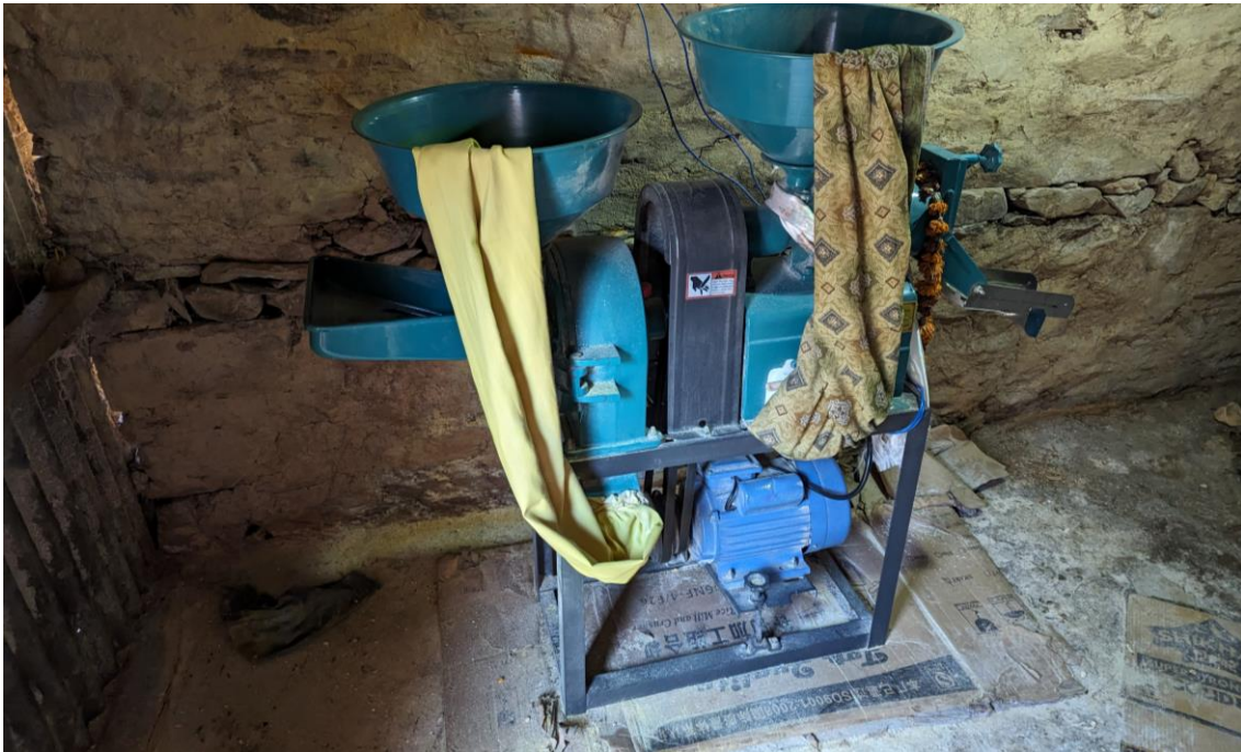
Figure 4: Rice mill that was used for de-husking and grinding rice and other grains (Own photograph)
