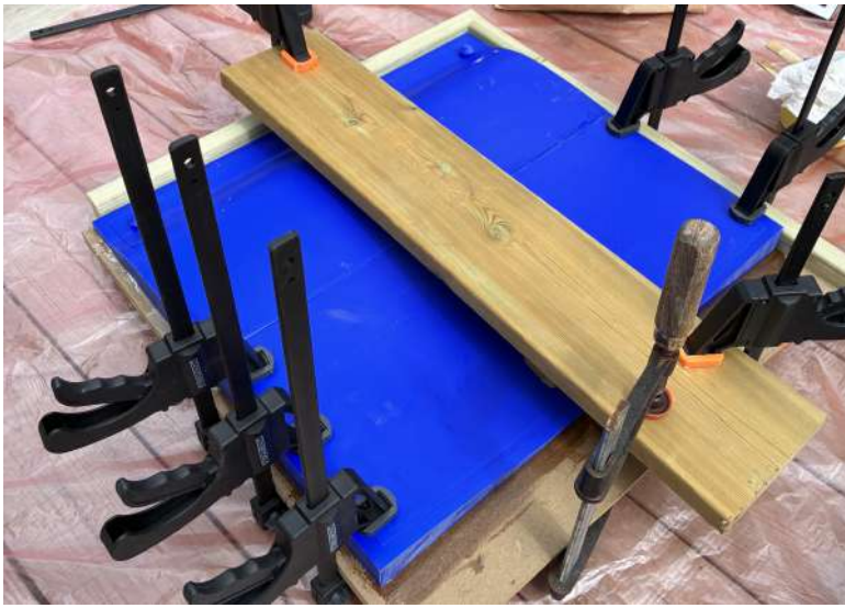
(a) Example of clamping setup when gluing two sections to finish one of the tool halves.
