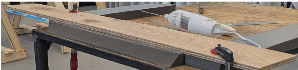
Figure 3.2: Angle cutting jig
