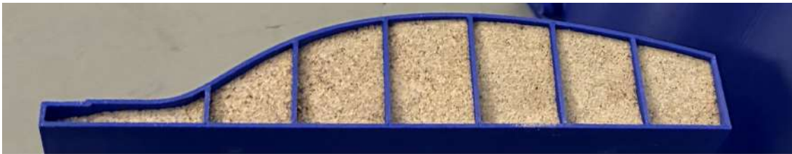
(a) Mould after cavities have been filled with sand.
