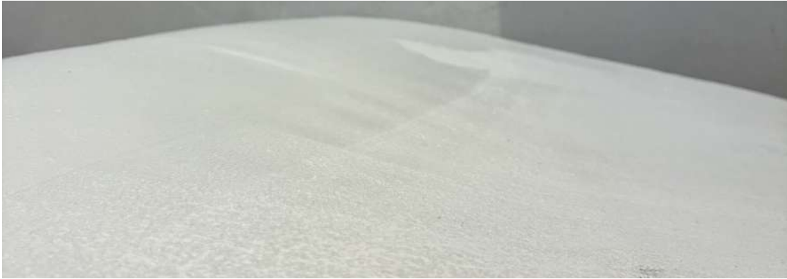
Figure 4.1: Foam where the right side of the surface has been surface and has a rugged finish and the left side has not been sanded and has a slippery finish.
