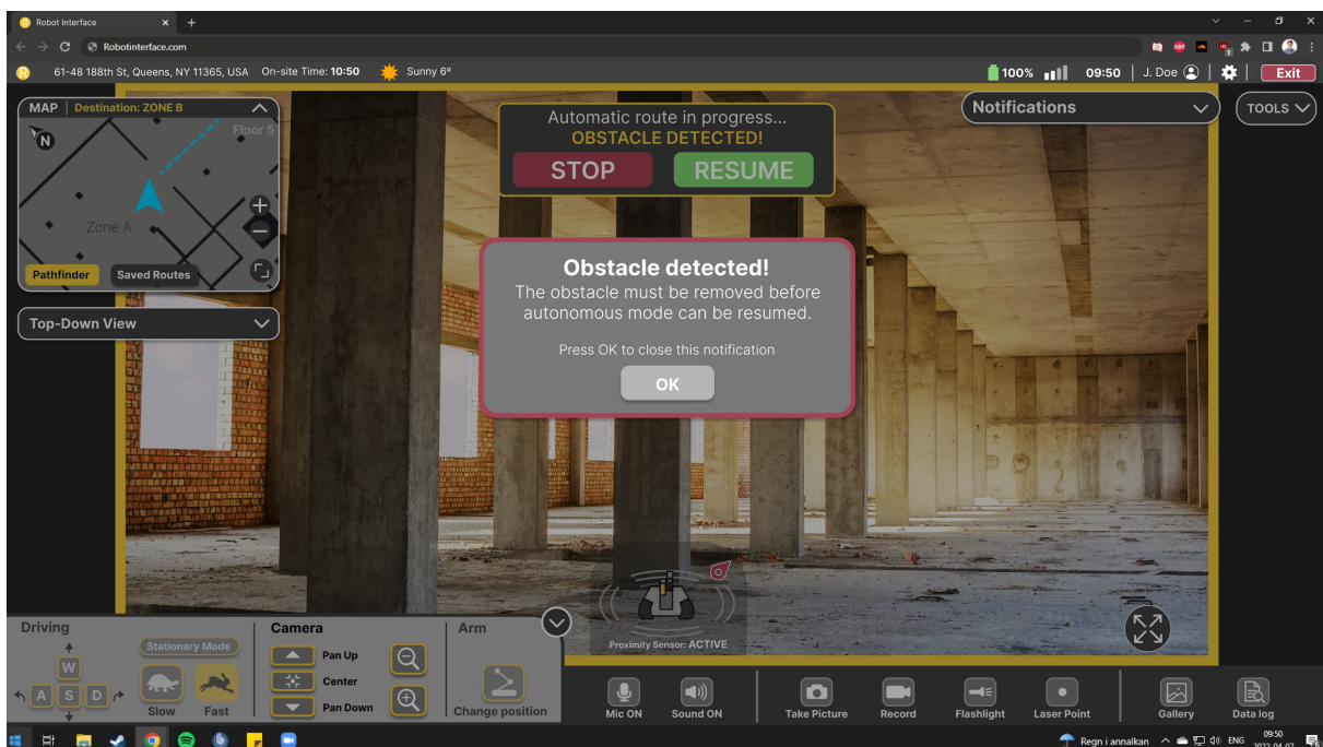
Figure 27: Interface with notification alerting that an obstacle has been encountered.
