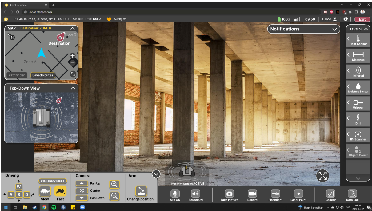
Figure 12: The main page with expanded top-down view and tools panel.
