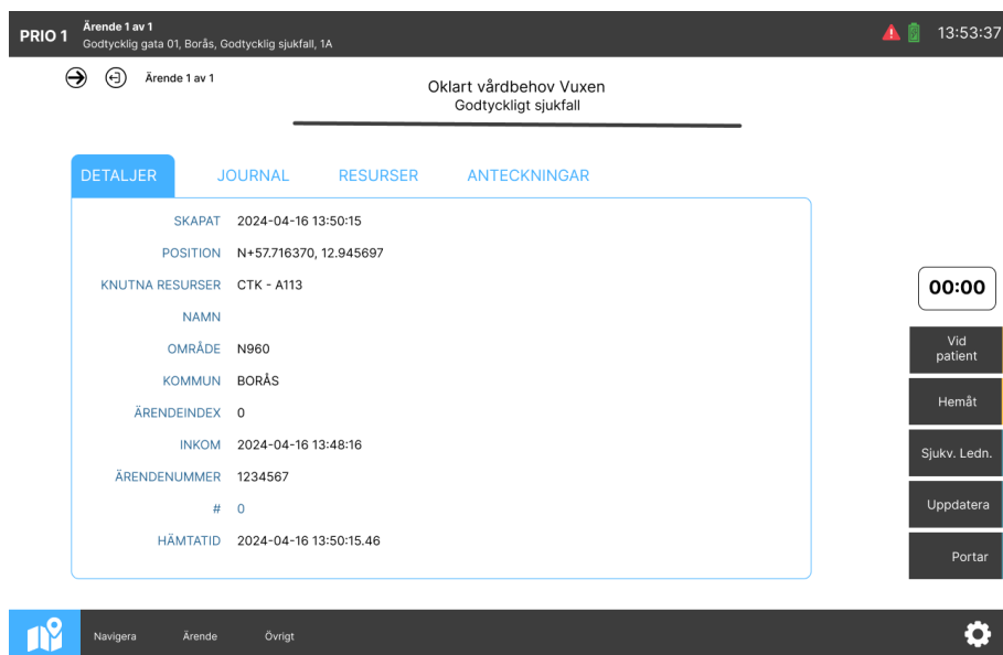
Figure 4.19: The default view of the second terminal that is taken with to the patient. Displaying the mission information, medical records, other connected resources and notes.
