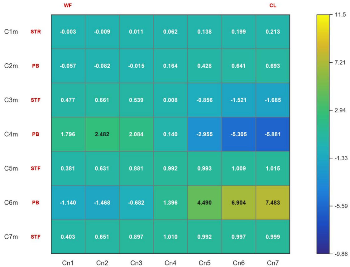
Figure 39 Normal-strain measurement for the 400 mm (transverse) \times 800 mm (longitudinal) C-series patches.
