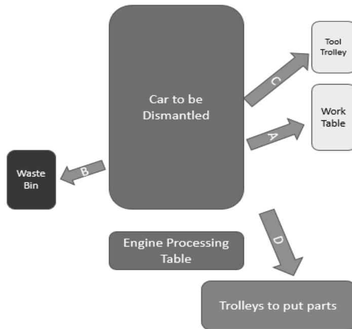
Figure 13 Layout and Movement diagram of operator in dismantling station
