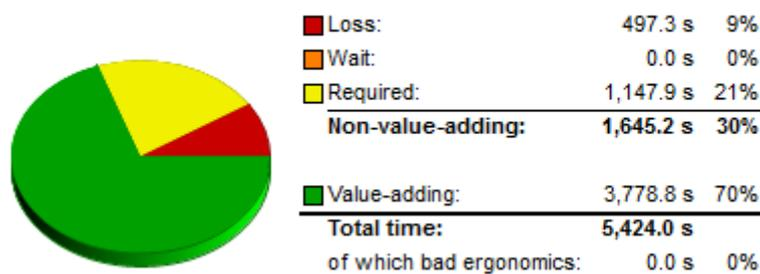
Figure 12: Summary result of task analysis in dismantling station
