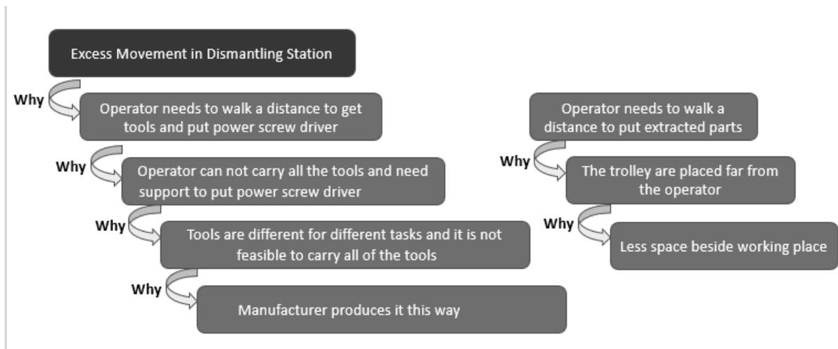
Figure 15: Five-Why analysis of Excess movement of operator in dismantling station
