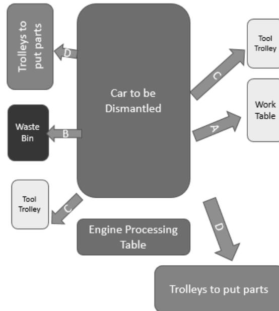
Figure 16: Improved Layout and movement path of operators in dismantling station
