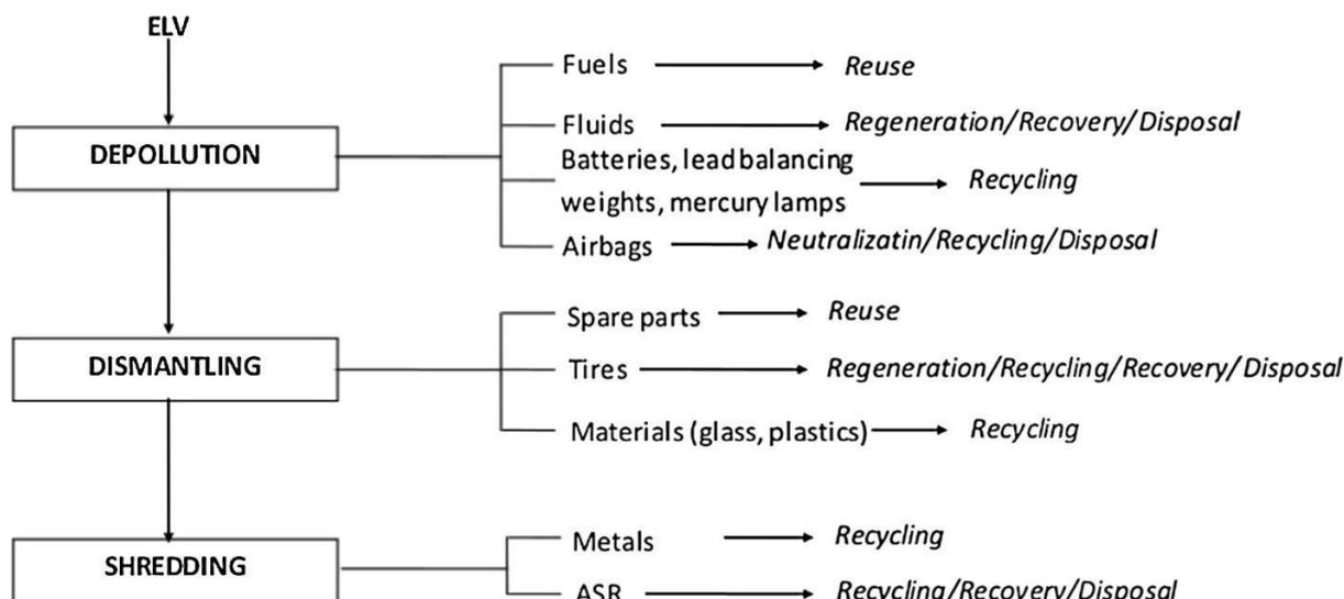
Figure 2: Production Processes in dismantling company (Cossu & Lai, 2015)
