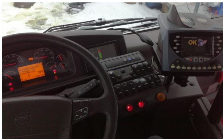
Figure 1: How the on-board computer and other systems are placed in a driver cabin
