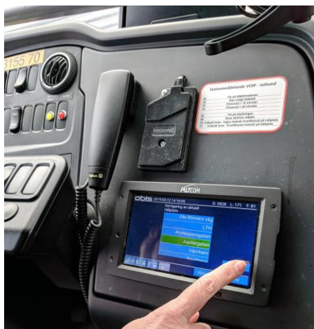
Figure 3: How an on-board computer is placed and its text size
