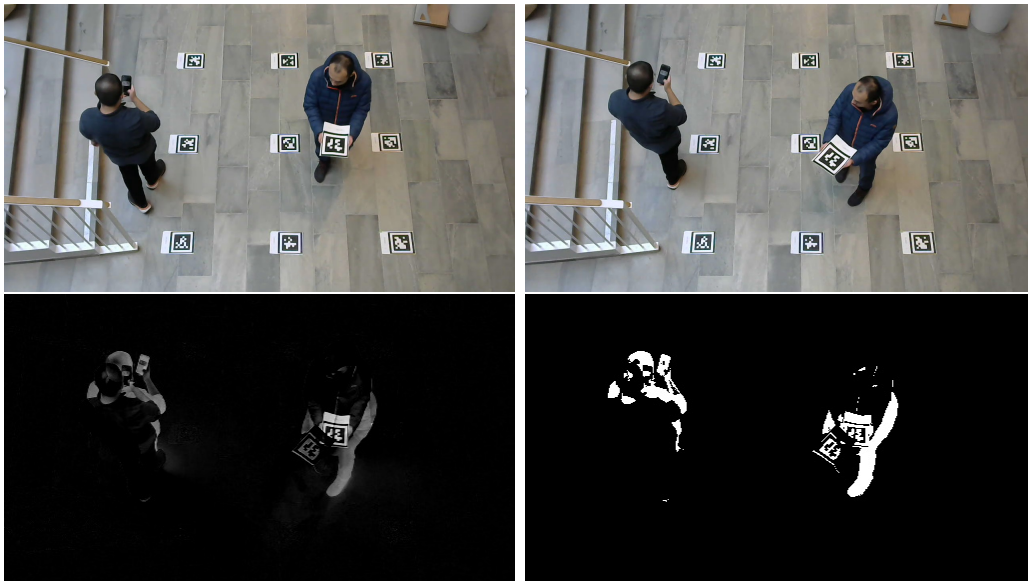
Figure 3.5: Frame Subtraction performed on a frame and a previous frame a) Empty floor b) Current frame c) Difference in frames d) Thresholding performed on the difference frame
