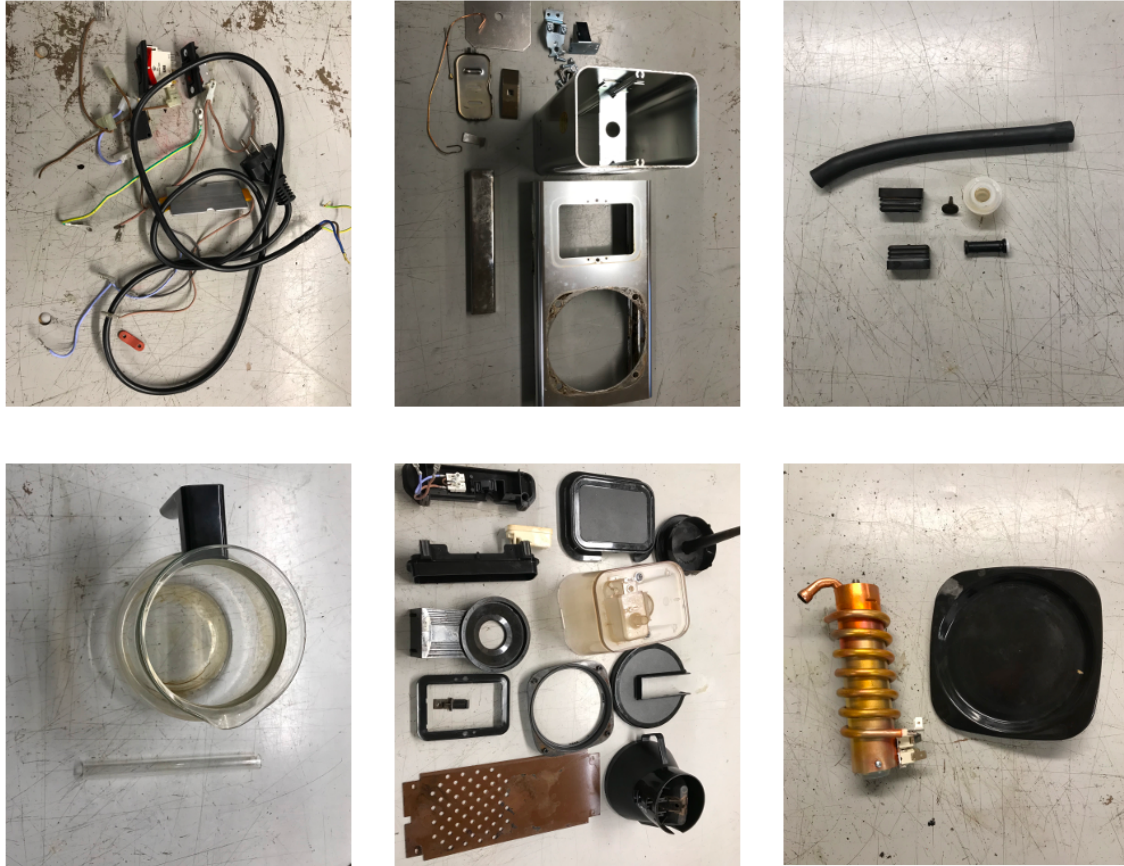
Figure 7.9: Top left: Electronics. Top middle: Metal. Top right: Rubber. Bottom left: Glass. Bottom middle: Plastic. Bottom right: Other (Hot plate and heat exchanger).
