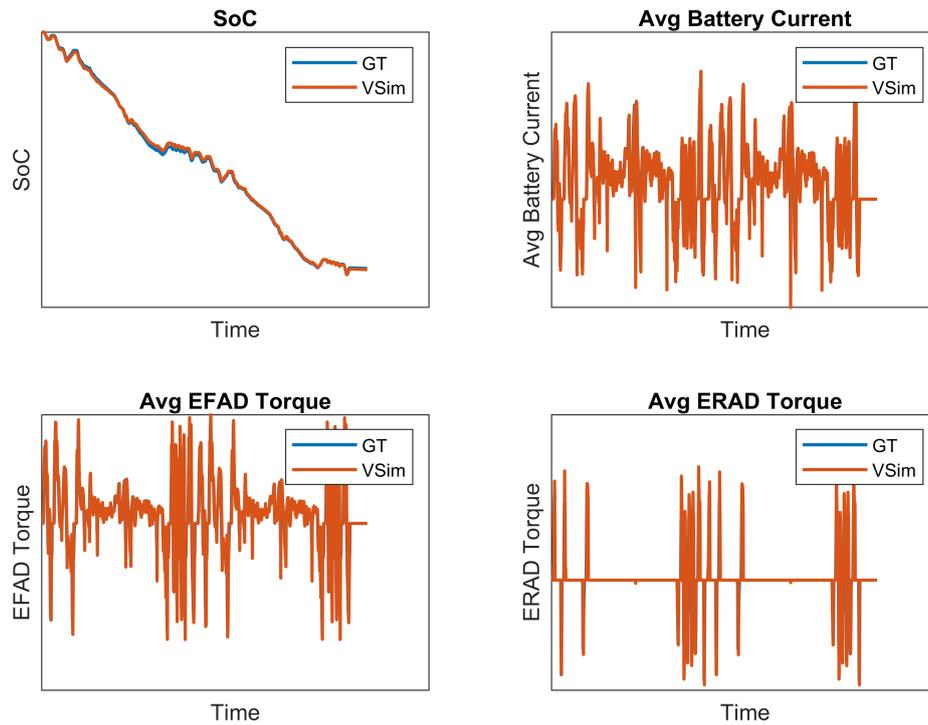
**Figure 4.1:** Comparison for US06 drive cycle at 25<sup>0</sup>C (normalized to GT-Suite)
