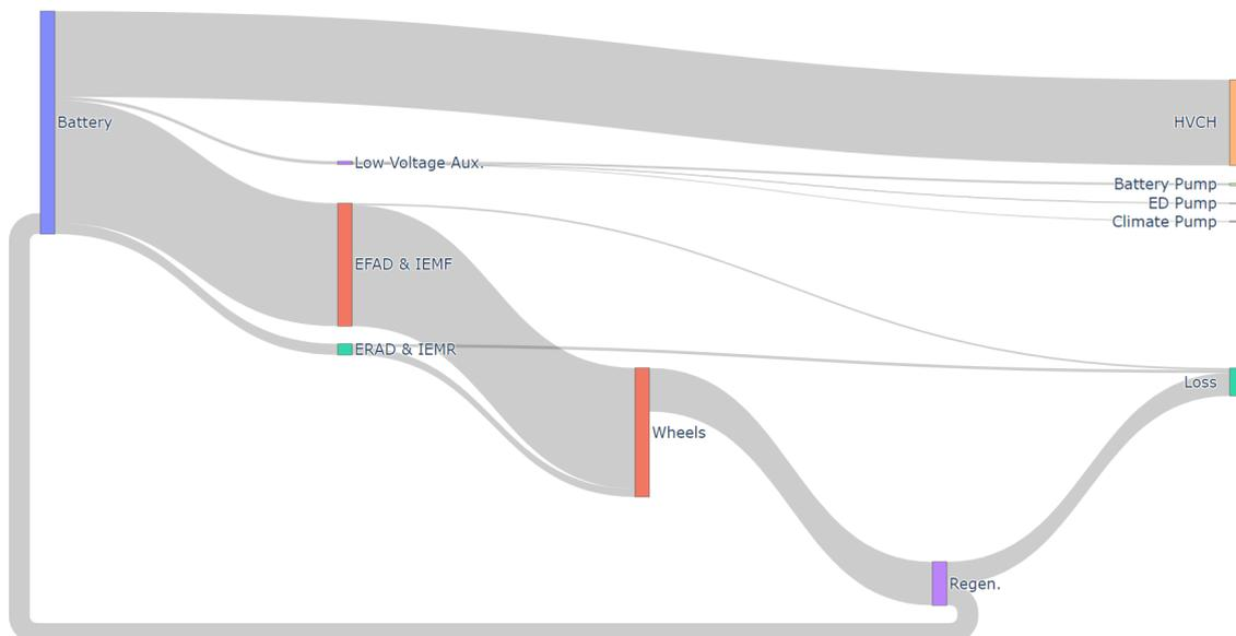
**Figure 4.12:** Sankey diagram for WLTC at  $-7^{\circ}\text{C}$
