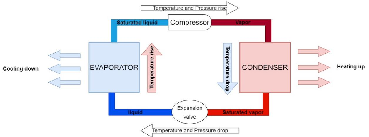
Figure 2.12: Refrigerant circuit
