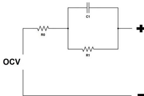
**Figure 2.9:** Thevenin equivalent circuit with a single RC branches
