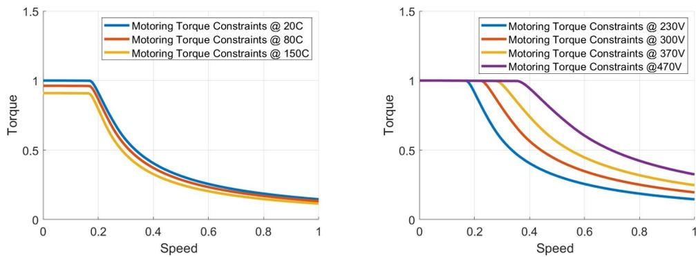
**Figure 2.5:** Electric machine constraints on temperature and voltage (normalized axes) [1]
