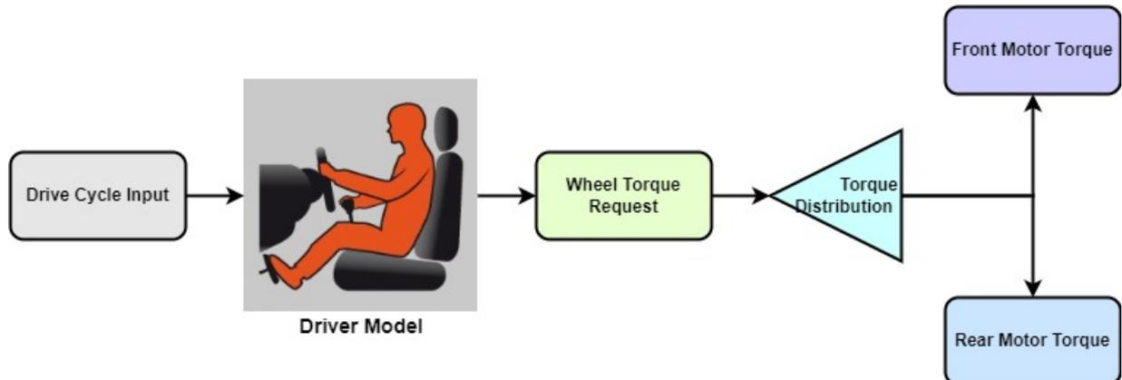
Figure 3.6: Torque control
