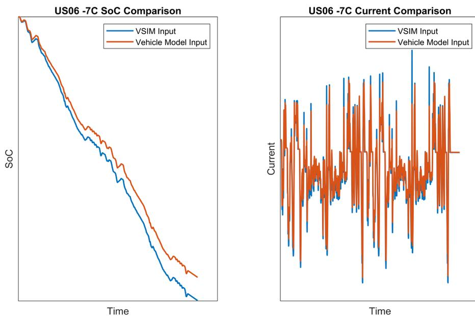
**Figure 4.5:** Comparison for US06 drive cycle at  $-7^{\circ}\text{C}$  (normalized to GT-Suite)
