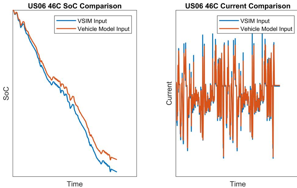
**Figure 4.4:** Comparison for US06 drive cycle at  $46^{\circ}\text{C}$  (normalized to GT-Suite)
