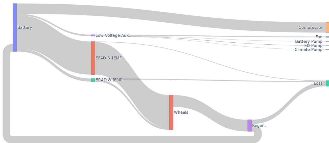
**Figure 4.13:** Sankey diagram for WLTC at 35<sup>0</sup>C
