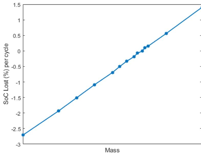
**Figure 4.10:** Battery energy consumption with variation in mass per WLTC cycle
