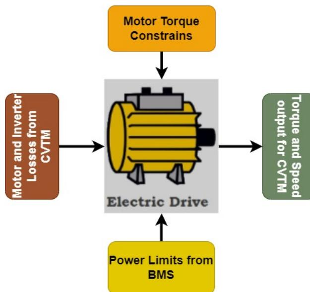
Figure 3.8: GT-Suite electric motor model
