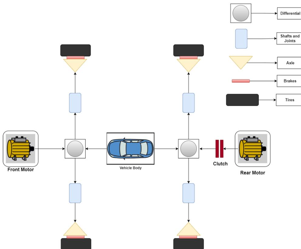
**Figure 3.2:** All wheel drive vehicle chassis component
