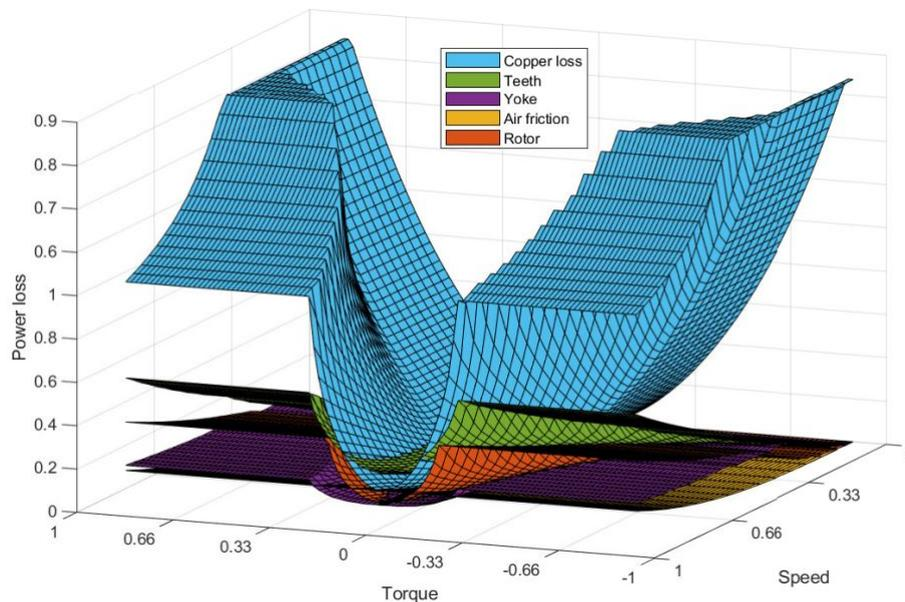
**Figure 2.6:** Electric motor component losses [6]
