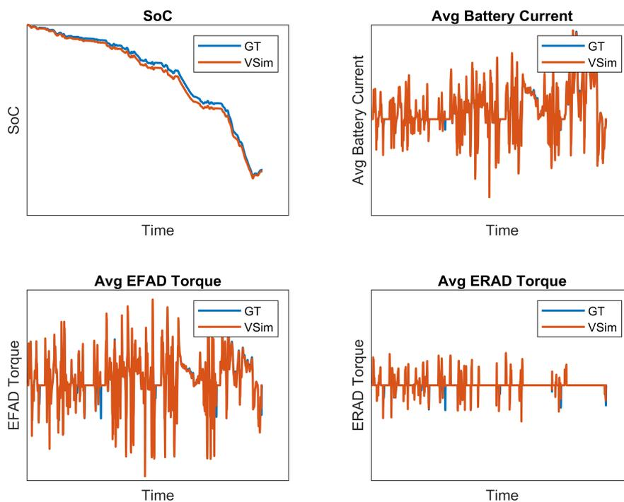
**Figure 4.3:** Comparison for WLTC drive cycle at 25<sup>0</sup>C (normalized to GT-Suite)
