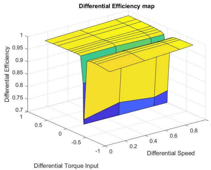
**Figure 2.4:** Differential efficiency map[1]
