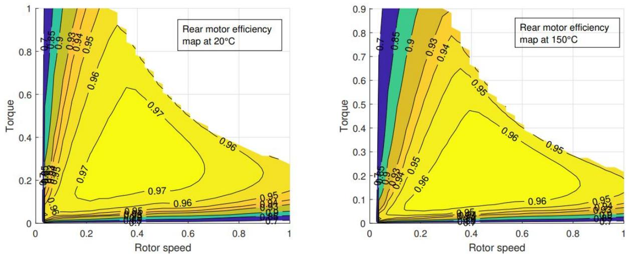
Figure 2.7: Electric machine efficiency map [6]
