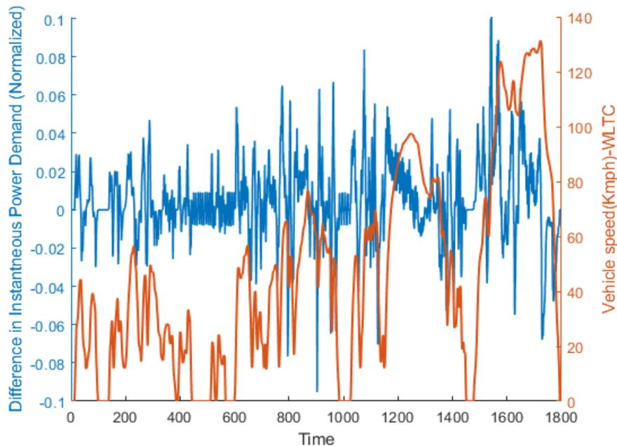
**Figure 4.11:** Normalized instant power demand for a mass difference of 300kg
