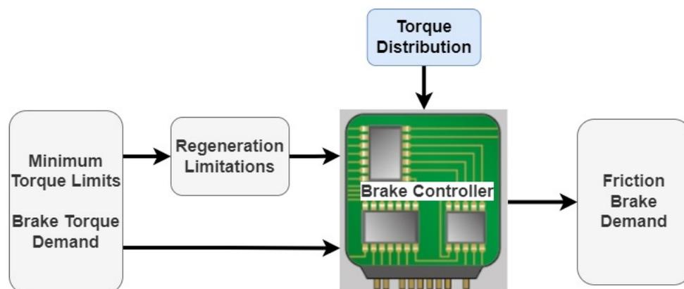
Figure 3.7: Brake controls
