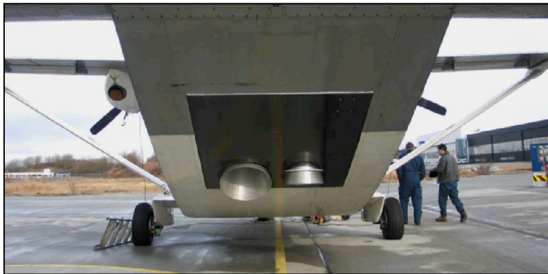
Figure 18: EMIRAD horn antennas mounted on the Skyvan
