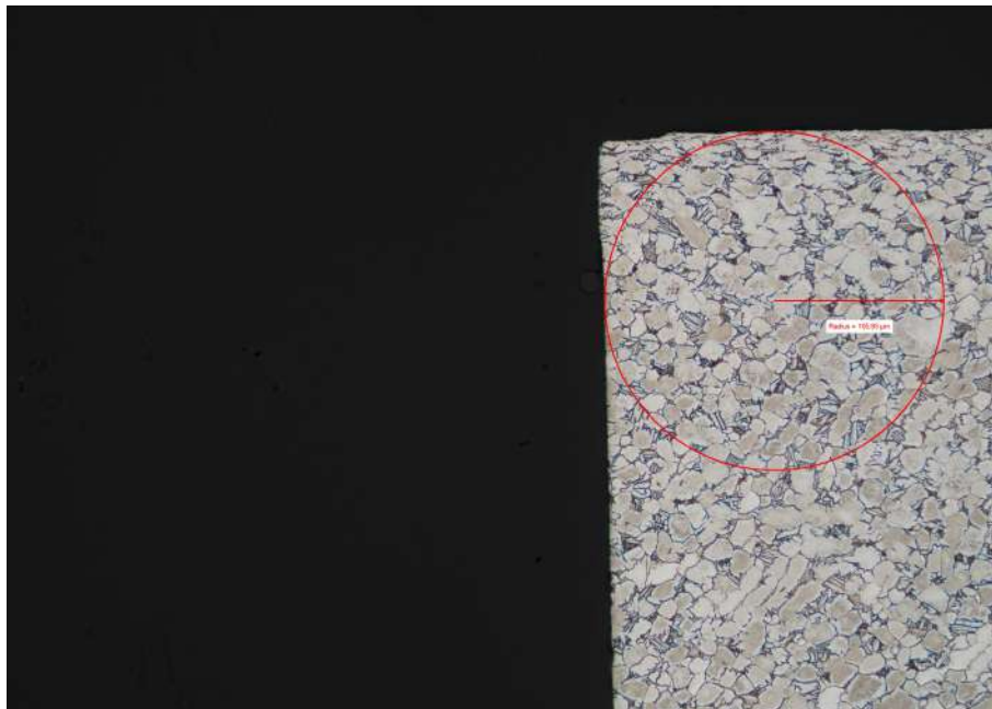
Figure 5.1: Photograph of the top left corner of the cross-section used for the validation of test piece geometry. Captured with the 5X objective.
