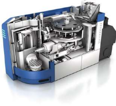
Figure 4.6: A illustration showing the layout of a GROB G350 [29]
