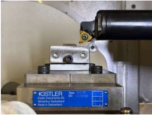
Figure 4.8: Photograph of how the test piece, machine vise, and Kistler sensor are positioned.
