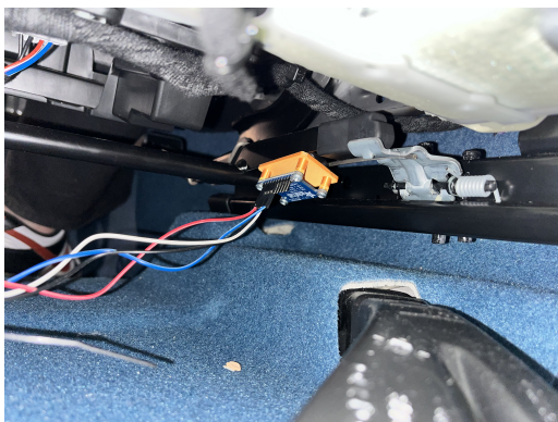
Figure 3.3: Accelerometer attached with magnets under Volvo EC40 driver seat
