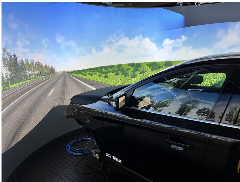
Figure 1.2: Interior of Sim IV with Volvo XC60 cabin
