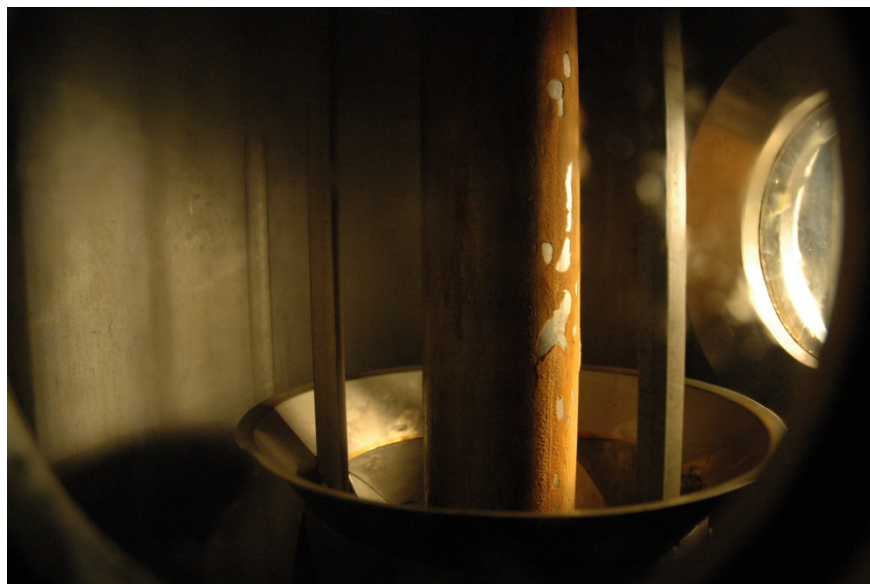
Figure 5-15. Fouling on the tube after experiment 3.
