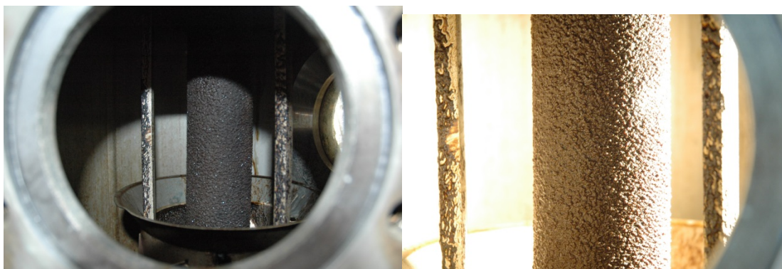
Figure 5-18. Thick fouling layer after the long experiment 6, from 6.5 % to 30 % ds
