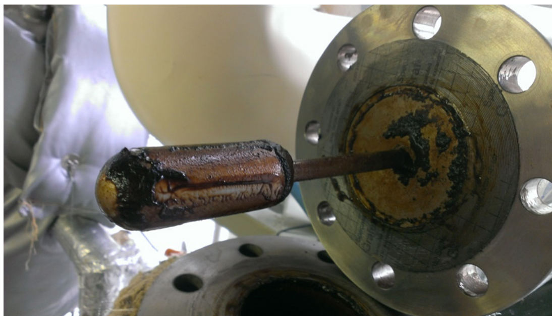
Figure 4-2. Fouling of the viscometer after experiment 5
