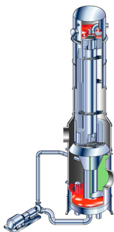
Figure 3-3. The structure of a falling film evaporator where the solution flows on the outside of the tubes (Metso Power AB, 2013).
