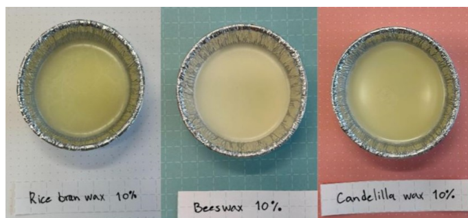
Figure 4.2: Overview of constructed oleogels with 10% w/w of rice bran wax (RBW10), beeswax (BW10) and candelilla wax (CW10).
