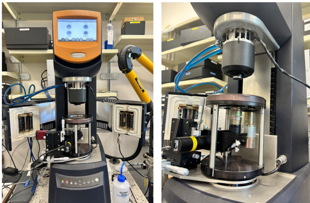
Figure 3.1: Images of the HR30, hybrid rheomicroscope, used for the rheological and microscopic measurements.
