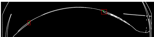
(c) Nominal fisheye right camera. Green points are the optimal points. Red rectangles are the template regions.
