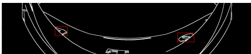
(a) Nominal fisheye back camera. Green points are the optimal points. Red rectangles are the template regions.
