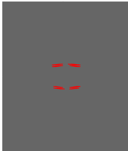
Figure 4.10: Crack stress and strain of top surface at load 19.7 \text{ kN/m}^2 (first crack at top surface).
