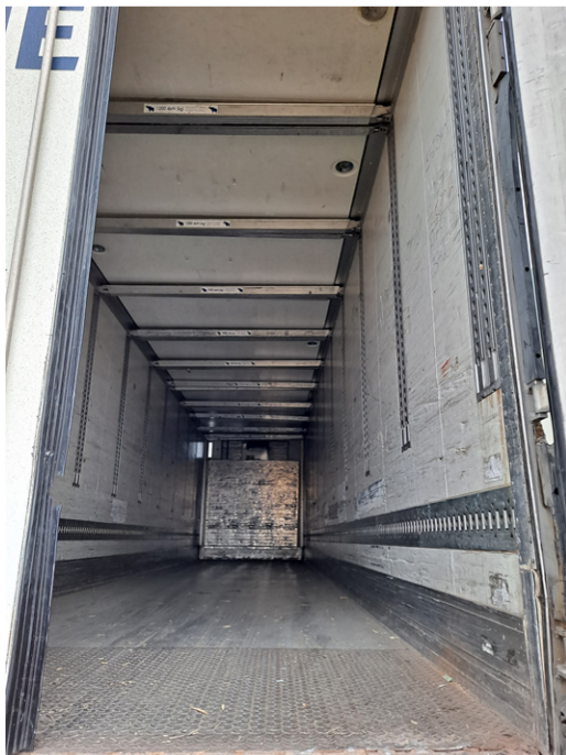
Figure 4.10: Bars are located in the ceiling of the carriage when not used.
