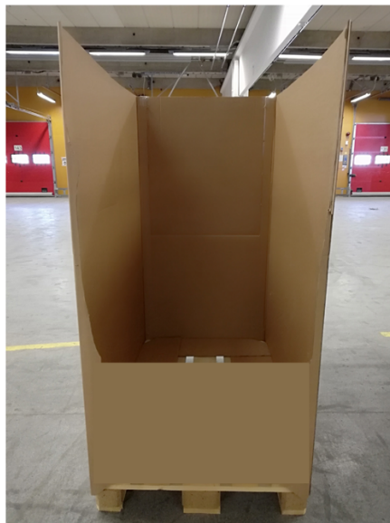
Figure 1.7: The corrugated cardboard cage used when shortage of parcel-cages occurs.
