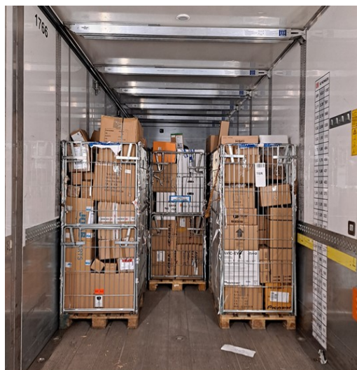
Figure 1.6: Cages loaded into a carriage with the gap in height between the cage's top and the ceiling of the carriage visible.
