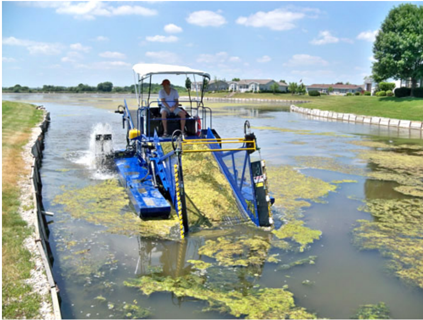
Figure 5.9: Harvester with conveyor belt (Aquarius Systems, 2010)
