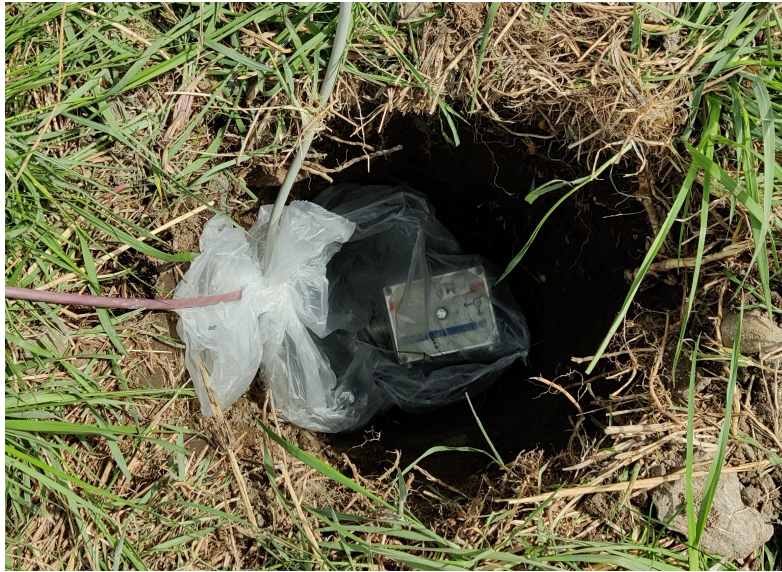
Figure 4.3: Geophone placed in a hole in the ground at Åsa station. After the unit has been leveled the hole is carefully refilled with soil and is then ready for operation.
