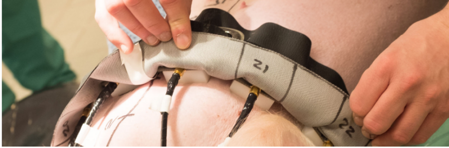
Figure 3.1: The microwave belt attached around the thorax of the pig.
