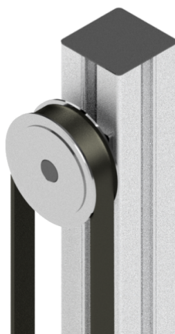
Figure 7.6: A closeup of one of the pulleys and the belt
