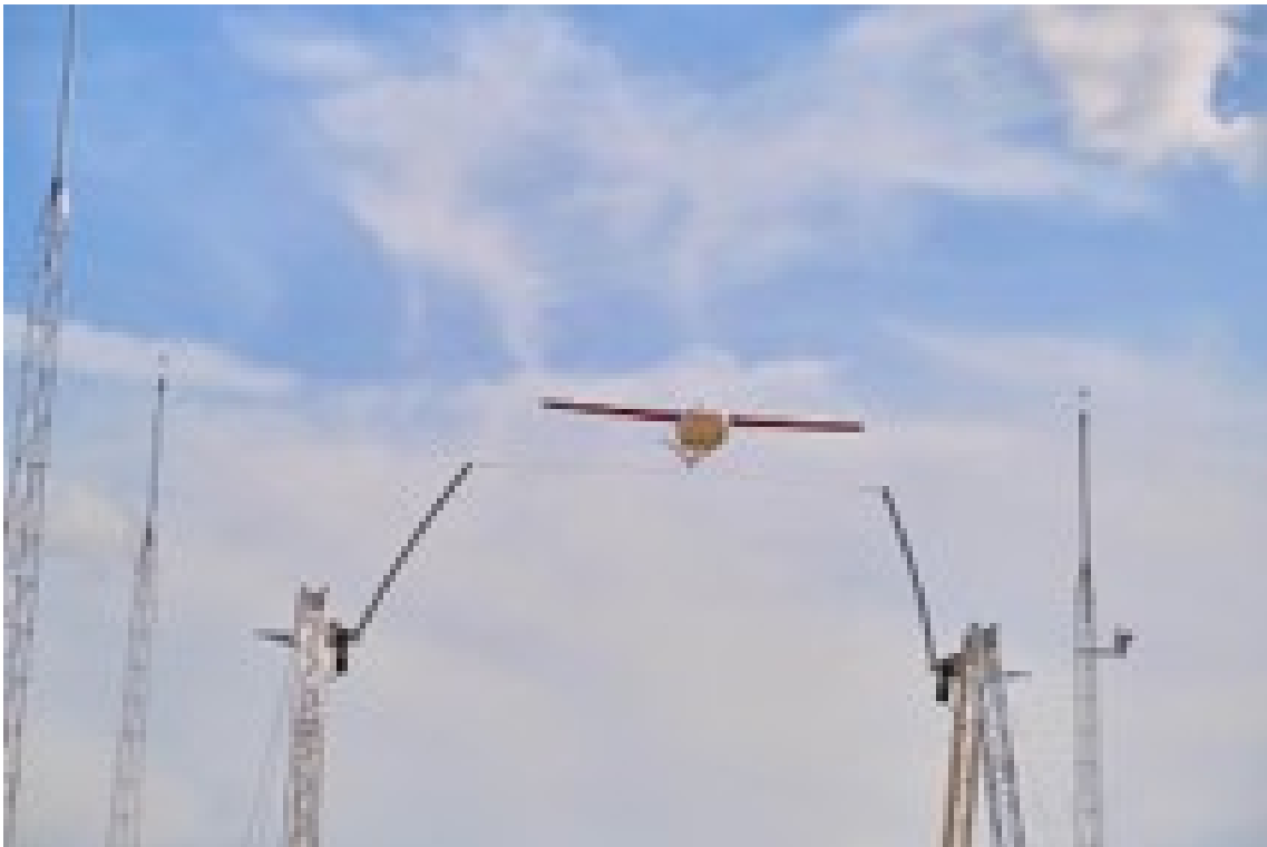
Figure 4.1: Zipline's hook-based recovery method [22]
