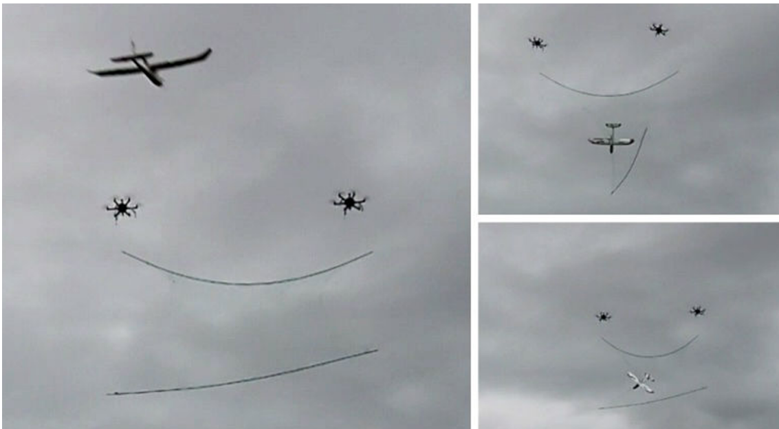
Figure 4.3: Net-based recovery method using two multirotor UAVs [25]
