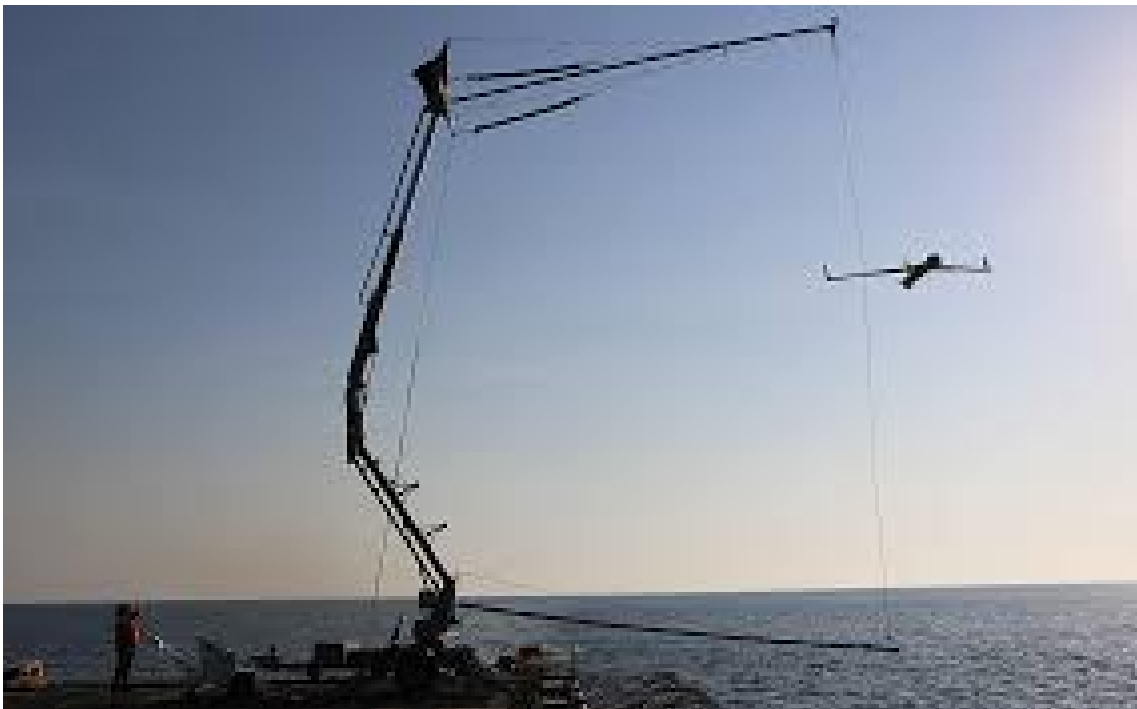
Figure 4.2: Insitu's hook-based recovery method [24]
