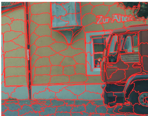
Figure 1.1: Superpixels generated by the untrained superpixel sampling networks, SSN-pix [4], on an image from the Cityscapes dataset [1].
