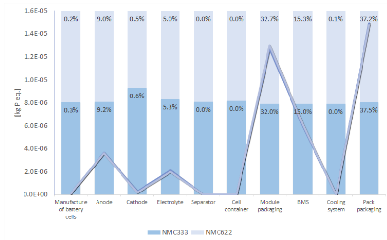
Figure 5.8: Contribution of different components and processes to the cradle-to-gate environmental impacts on freshwater eutrophication for NMC333 and NMC622. The right axis represents the absolute value whereas the left represents shares of the total impact on freshwater eutrophication.
