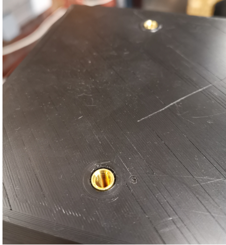
Figure 5.4: M6 screw insert melted into the upper middle part of the bus model
