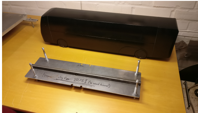
Figure 5.13: The adapter between the scale and the bus wheels
