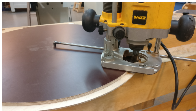
Figure 5.14: Cutting out an edge on the rotating plate with the router
