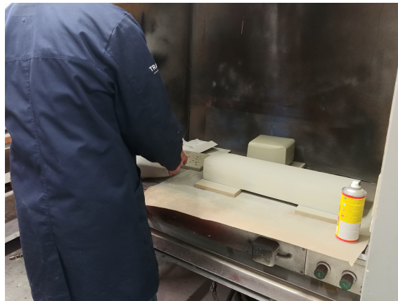
Figure 5.7: The bus model with spray filler applied
