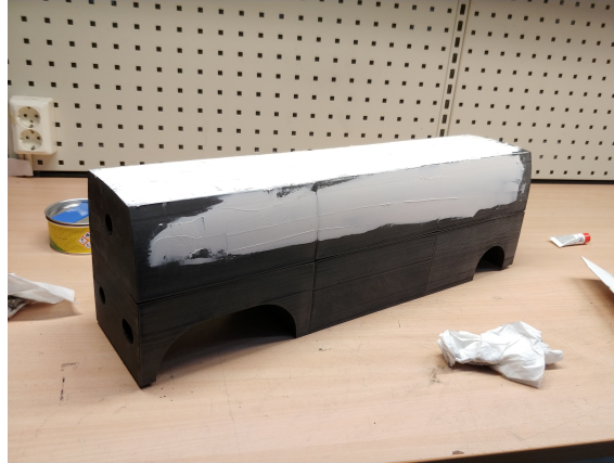
Figure 5.6: Part of the bus model where filler have been applied
