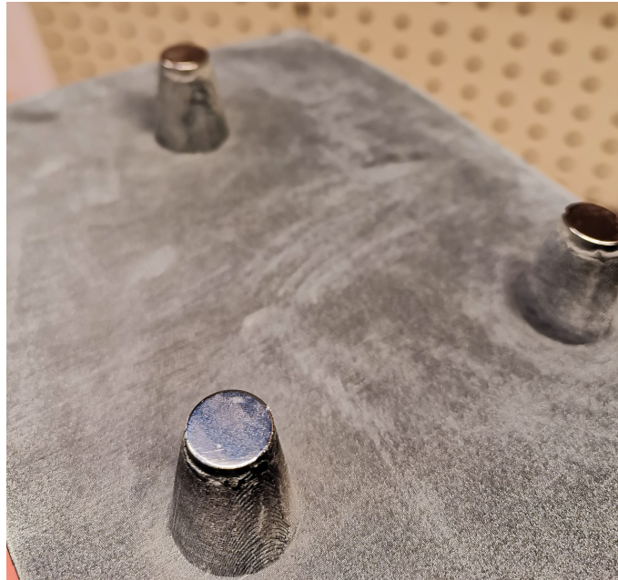
Figure 5.5: The magnets that hold the front and rear part together with the center of the bus
