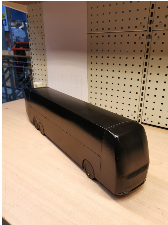
Figure 5.9: Assembled bus model with completed surface treatment
