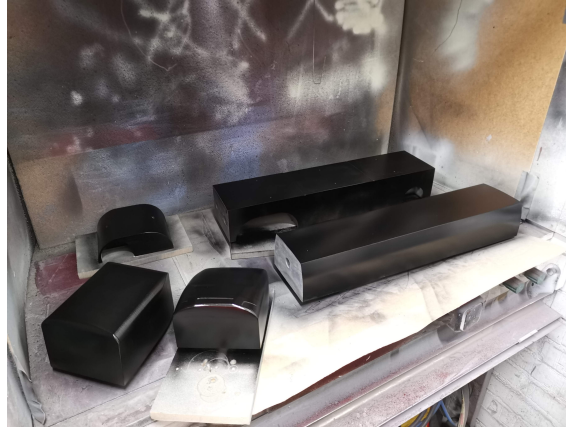
Figure 5.8: Parts of the bus model with paint applied
