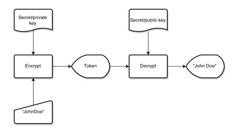
Figure 4.2: Illustration of how a string is encrypted and decrypted using either a secret or private/public key architecture.
