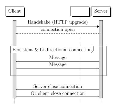
Figure 4.3: WebSocket sequence diagram.
