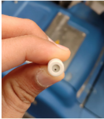
Figure 3.2: Drilled hole of 1 mm inside the plug.
