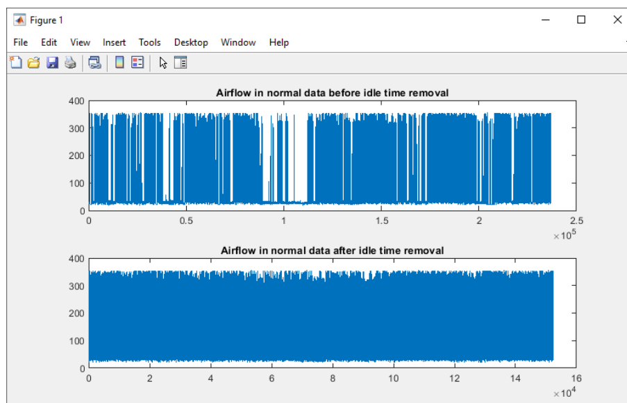
Figure 4.8: Comparison of airflow before and after idle time was removed for normal data.
