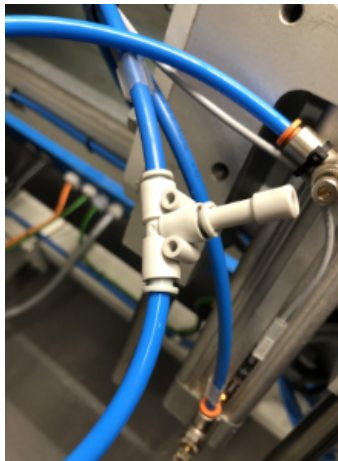
Figure 3.3: Tee tube-to-tube adapter with plug and a small drilled hole.
