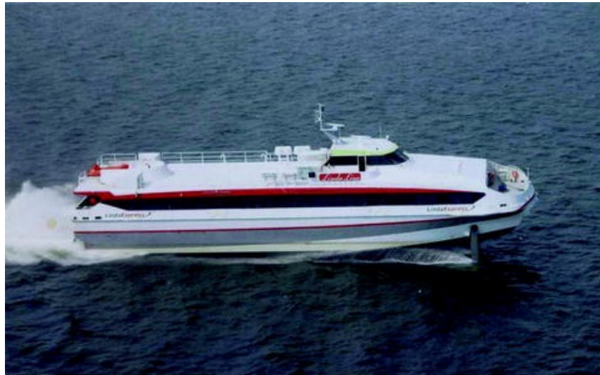
Figure 5.4: The Superfoil40 passenger ferry is a foil assisted catamaran. Adopted from Yun and Bliault (2012)
