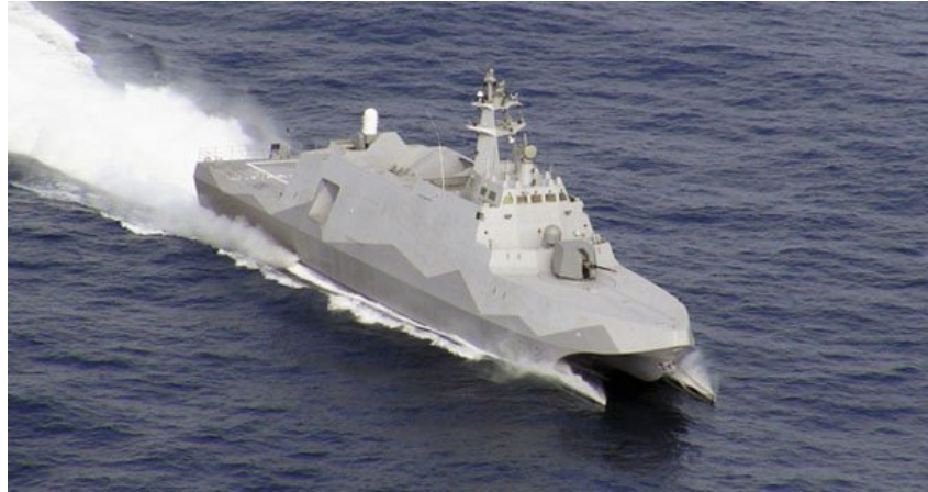
Figure 5.2: The South Korean Tuo Chiang-class corvettes is an example of a catamaran design. Adopted from Teh (2019)
