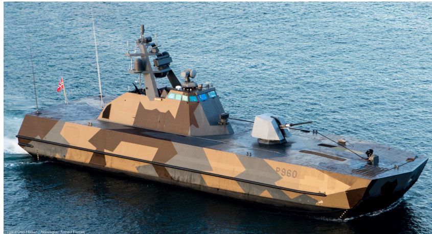
Figure 5.5: The Norwegian Skjold-class is a Surface Effect Ship. Adopted from Forsvaret (2023)
