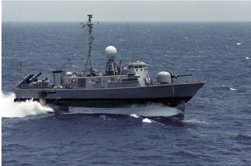
Figure 5.3: The American Pegasus-class was a class of fast patrol craft fitted with hydrofoils. Adopted from Hurst
