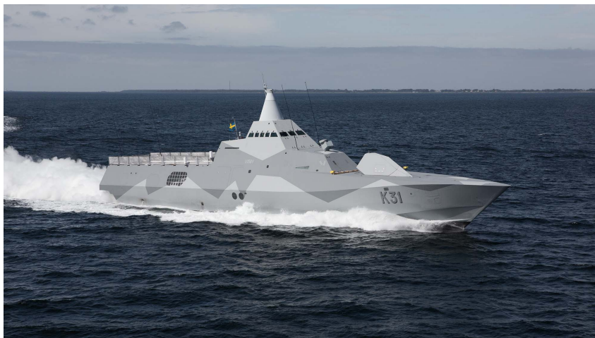
Figure 5.1: The Swedish Visby-class corvette is an example of a monohull design. Adopted from FMV (2025)
