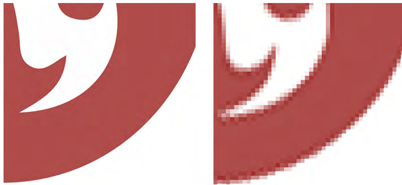
Figure 4.6: Zoomed in details of a vector image(left) vs raster image(right). Image created by the authors.
