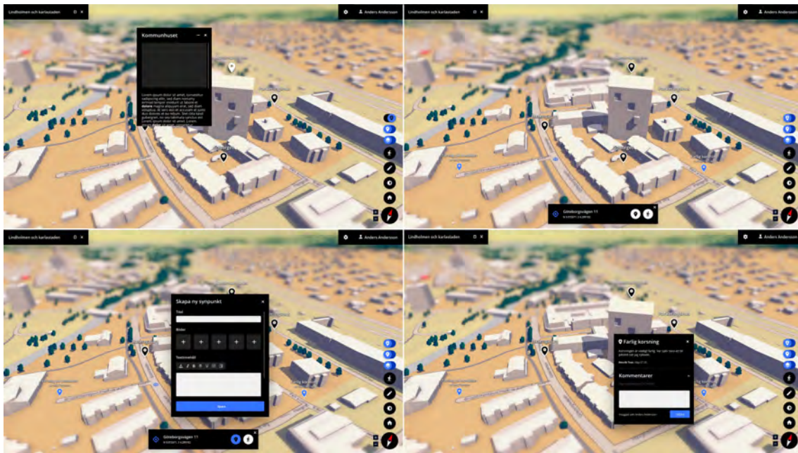
Figure 6.3: Project view . Top left: Active point of interest, displaying in a floating window. Top right: Marked position, positional options pane active. Bottom left: Create new point of interest on position. Bottom right: User made point of interest, displaying in floating window.
