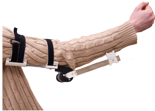
Figure 6.3: The elbow orthosis without sensors mounted. Note how the motor ends up below the elbow.
