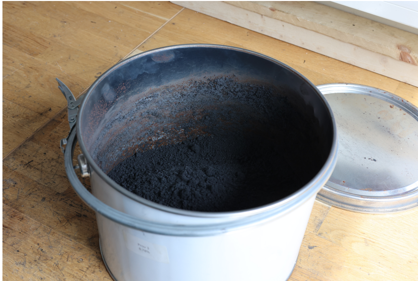
Figure 6: Container with iron ore concentrate sampled from LKAB processing plant
