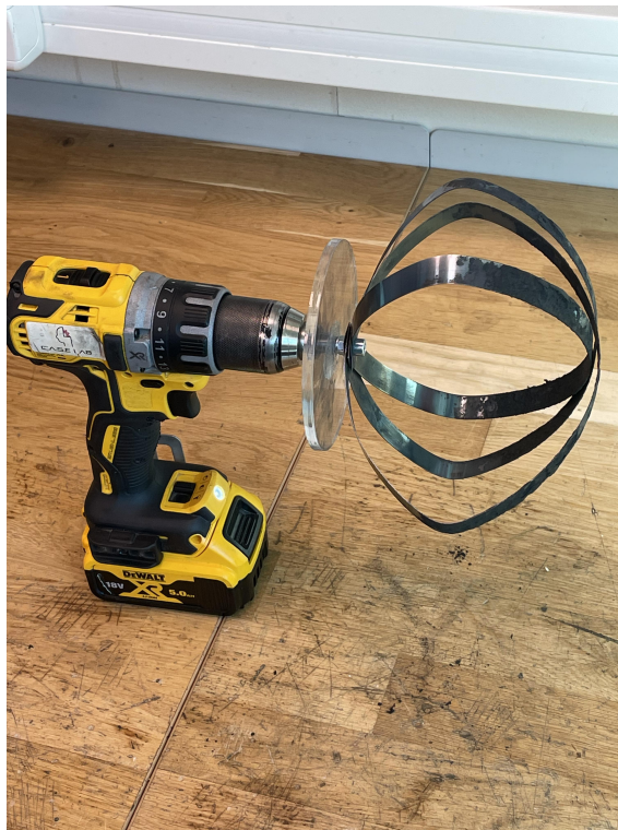
Figure 8: The device designed for mixing, crushing and homogenising iron ore concentrate
