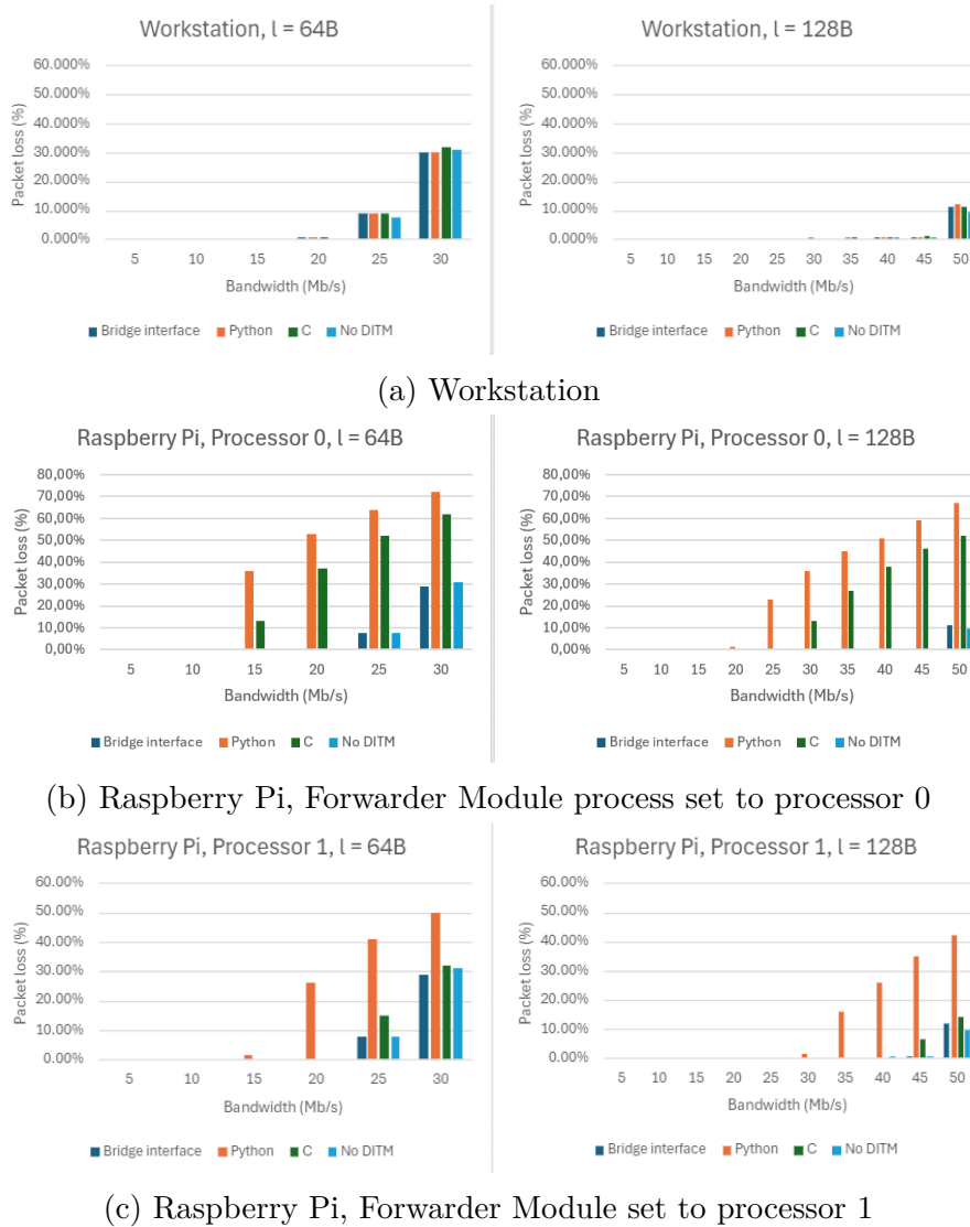
Figure 5.6: Performance testing results for the hardware and software setups compared to performance without DITM.
