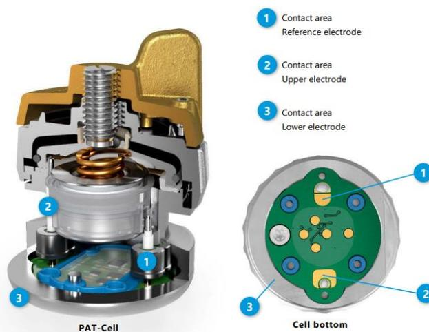
Figure 6. Description of a PAT-cell. Figure taken from [33].
