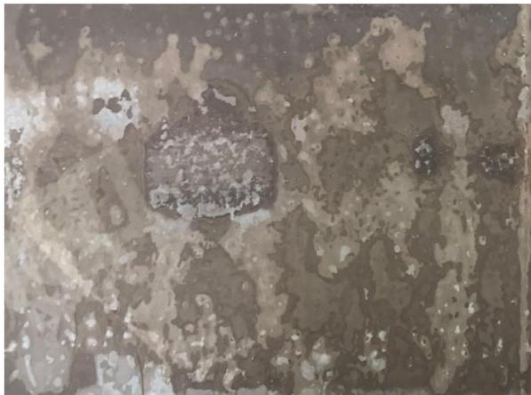
*Figure 15. Anode of cell 2 after 350 cycles, from second tear down.*
