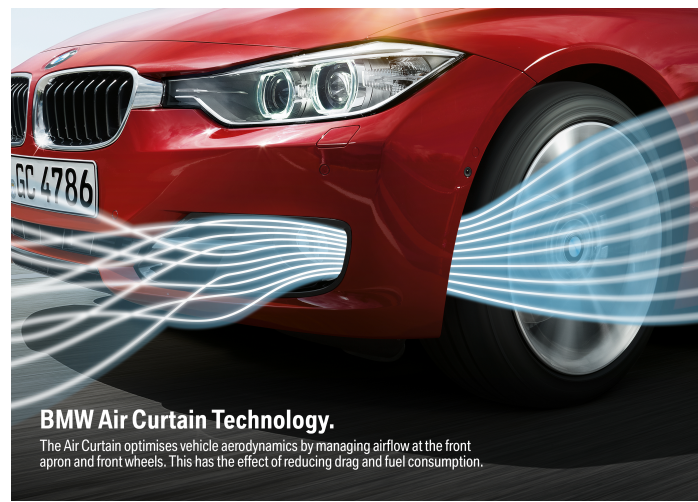
Figure 4.14: Indication of laminar flow created by air-curtains [27]
