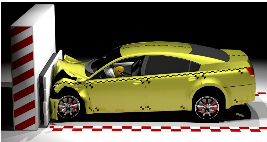
Figure 1.4: Frontal impact test[12]
